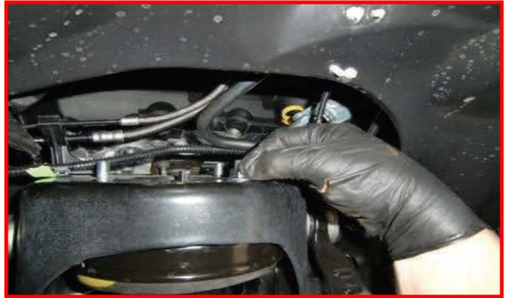
Raise the lower control arm up. Install the lower strut using the factory hardware. Do not tighten at this time.
