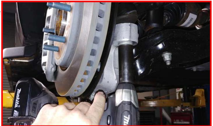
Remove upper ball joint from the knuckle. Strike the ball joint boss with a dead blow hammer to dislodge the taper.
