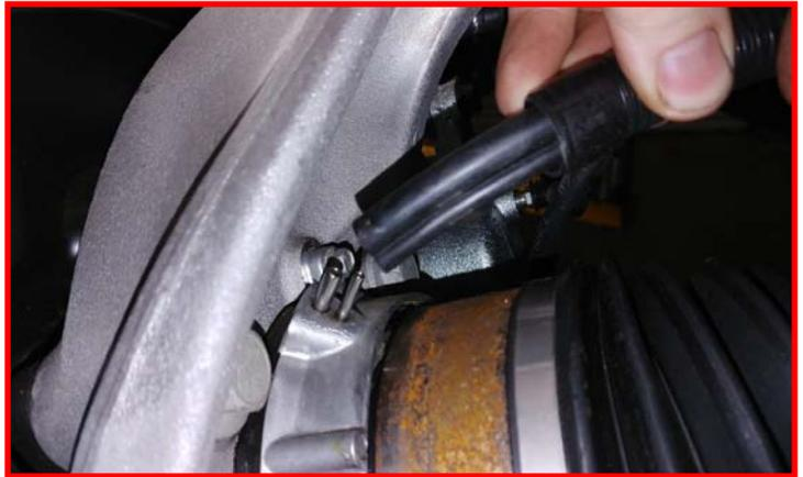
Remove the tie rod end at the knuckle. Use a dead blow hammer, strike the tie rod end boss to dislodge the taper.
