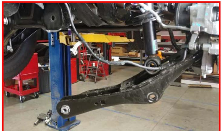
Locate the ReadyLIFT strut spacer. Install using the provided **M10 - 1.5 flange nuts**. Torque to **30 ft-lbs**. Install the completed strut assembly into the frame using the provided **M10 - 1.25 flange nuts**. Do not tighten at this time.
