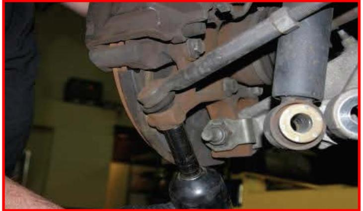
Remove the lower strut from the LCA.
