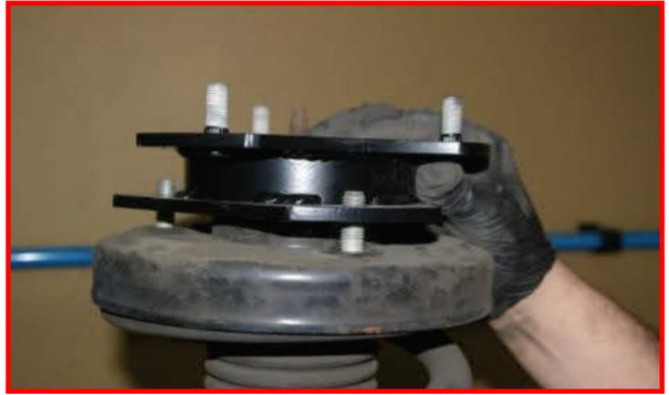
Install the completed strut assembly to the frame using the provided **M10 flange nuts**. Do not tighten at this time.
