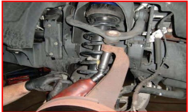
Attach the brake line/ABS bracket to the frame rail using the **factory hardware**. Do not over tighten as this is a self tapped hole and is easily stripped. Install the wheels and lower the vehicle to the ground. Torque the lug nuts to the wheel manufacturers specs. Jounce the vehicle to settle the suspension to the new ride height.
