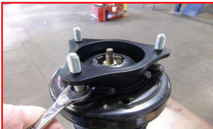
Install the strut to the frame using the provided M10 flange nuts. Do not tighten at this time.
