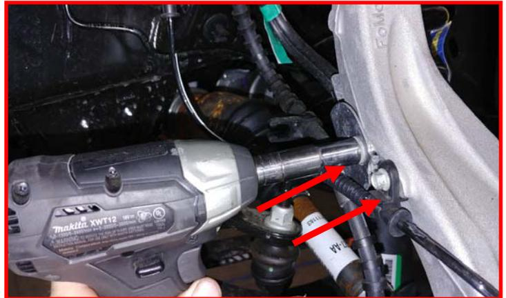
Install the **brake line bracket** to the frame rail using the **factory hardware**. Torque to **5 ft-lbs**. Install the ABS harness to the frame rail, brake line bracket, and rubber brake line using the factory clips.
