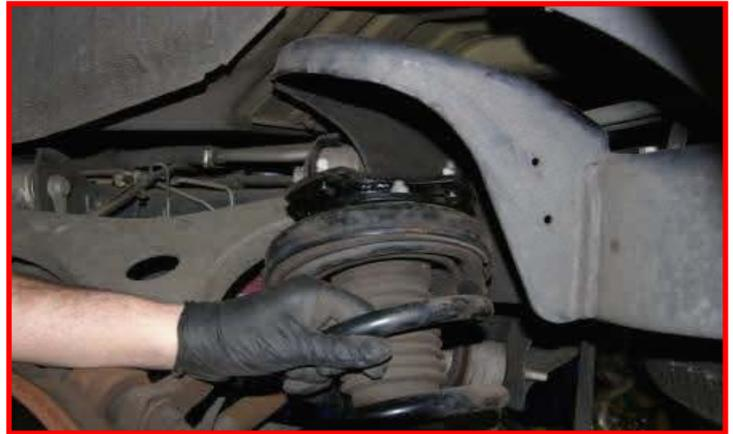
Raise the lower control arm and install the lower strut using the **factory hardware**. Do not tighten at this time. Install the tie rod end to the knuckle using the **factory hardware**. Torque to **45 ft-lbs**.
