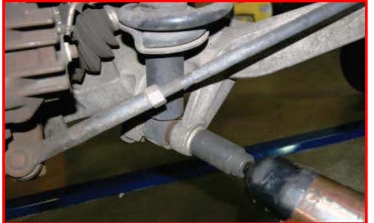
Remove the strut top hardware from the frame rail. Remove the strut from the vehicle.
