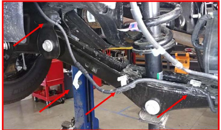
Loosen but do not remove all the trailing arm hardware at the frame and knuckle.
