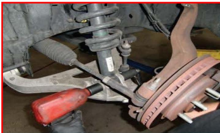
Remove the upper strut mount from the frame. Lower the LCA down while taking care to not over extend the brake lines and ABS wires. Adjust as necessary. Remove the strut from the vehicle.
