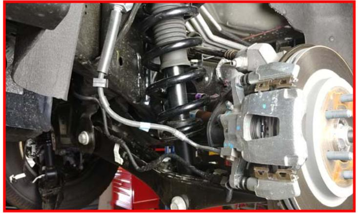
Remove the plastic clips from the control arm and frame rail. Let the ABS harness hang out of the way. Place a suitable jack under the lower strut mount.
