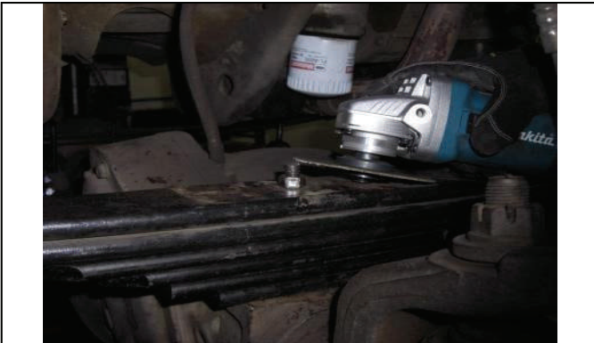
Cut-off excess threads to allow proper fitment of spring plate
