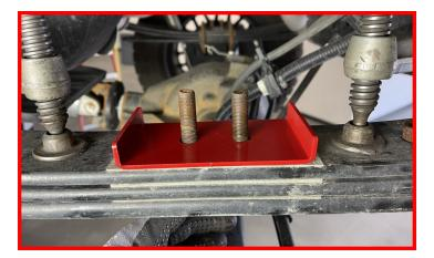
Install the leaf spring sensor spacer in the forward center pin using the factory nuts.
