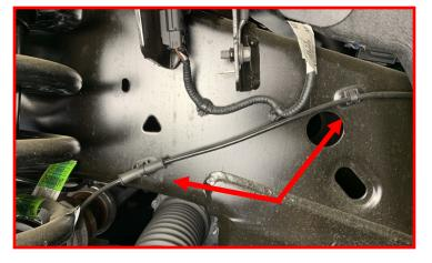
Connect the CCD solenoid harness connector.
