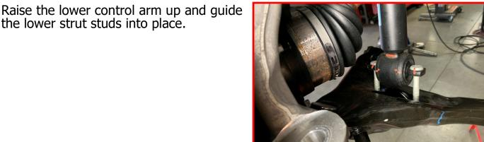
Continue to raise the lower control arm up until you are able to install the factory lower strut nuts.
