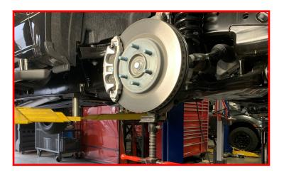
Remove the sway bar end link from the knuckle.
