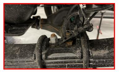
NOTE: IF VEHICLE IS EQUIPPED WITH CCD WITH LOAD SENSING (EXAMPLE OF SHOCK PIC-TURED) DO NOT INSTALL SUPPLIED SHOCK EX-TENSION.
