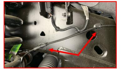
Connect the CCD solenoid harness connector.
