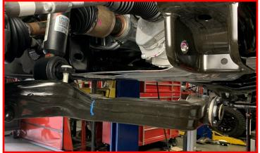
NOTE: USING A MARKING DEVICE LIKE A PAINT PEN, MARK THE STRUT AT THE OUTBOARD PO-SITION. THIS MARKING WILL BE MOUNTED IN-BOARD DURING LIFTED STRUT INSTALLATION.
