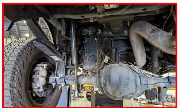
If equipped with a 2 piece driveline, remove the bolts holding the carrier bearing to the frame.
