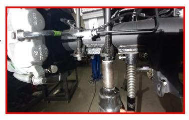
Lower the axle just enough to remove the factory block and install the ReadyLIFT block, making sure not to over extend brake and ABS lines. Adjust as necessary.
