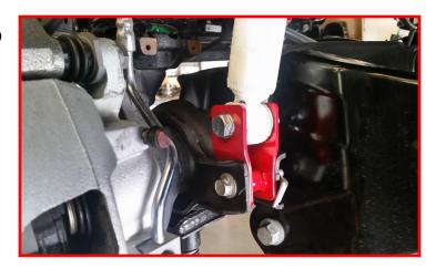
Install the factory brake line bracket at the axle using factory hardware.
