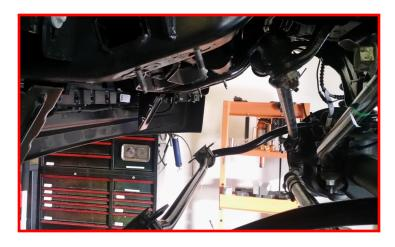
Lower the axle enough to remove the front springs. Install the ReadyLIFT urethane isolator, spring spacer, and then factory rubber isolator onto the spring.
