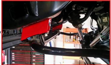
Install the ReadyLIFT shock extensions to the axle using factory hardware.
