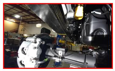
Locate the driver side lift block (Has a D cut into it under the bump stop tang). Raise the axle and the block up to the spring while aligning the center pin.
