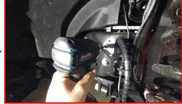
Remove the lower shock from the axle mount.
