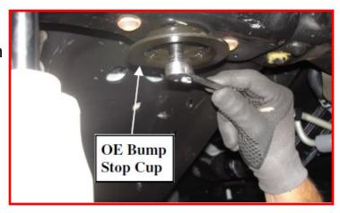
Install the **OE** bump stop cup to the bump stop extension using the supplied 8mm nut and washer.
