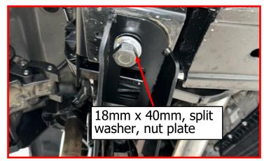
Carefully raise the radius arm into the drop bracket and secure it using the previously removed **OE** hardware.
