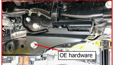
Install the supplied poly ring, coil spring spacer, **OE** isolator and coil spring.
