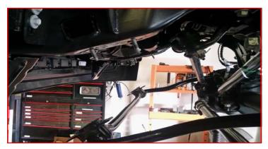
Remove the track bar from the factory bracket. Remove the factory track bar bracket from the frame.
