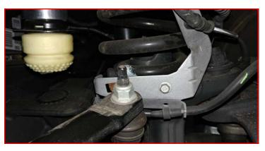
Install the ReadyLIFT brake line bracket to the factory brake line using 5/16" x 3/4" bolts, washers, and nuts. Install the bolt with the head between the bracket and the frame. Torque to 10 ft-lbs. Gently pull the metal brake line down while lining up the Ready-LIFT bracket to the original holes in the frame. Install using factory hardware. Torque to 5 ft-lbs.
