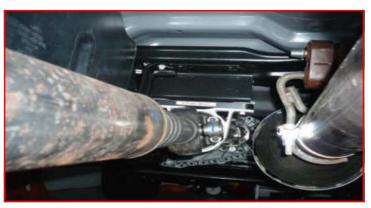
Lower the vehicle to the ground. Torque the lug nuts to the wheel manufacturer specs. Jounce the vehicle a few times to settle to the new ride height. Torque the u-bolts to 110 ft-lbs. Have a reputable alignment shop set the alignment to the factory specs.
