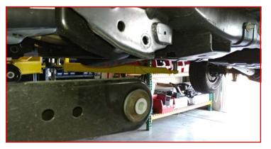
Install the ReadyLIFT radius arm drop brackets into the frame using M18 x 130mm bolts, washers, crush sleeve, and nuts. Do not tighten at this time.
