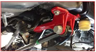
Lower the axle enough to remove the front springs. Install the ReadyLIFT urethane isolator, spring spacer, and then factory rubber isolator onto the spring. Raise the axle enough to hold the spring assembly in place.
