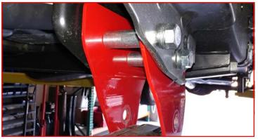
Rotate the axle until you can line up the radius arms into the ReadyLIFT drop brackets. Install using factory hardware. Do not tighten at this time.
