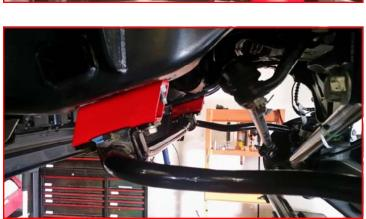
Install the ReadyLIFT shock extensions to the axle using factory hardware. Install the shock to the ReadyLIFT shock extensions using the M14 x 70mm bolt, washers and nuts. Torque to 45 ft-lbs.
