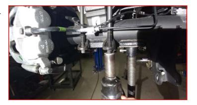
Lower the axle just enough to remove the factory block and install the ReadyLIFT block, making sure not to over extend brake and ABS lines. Adjust as necessary.
