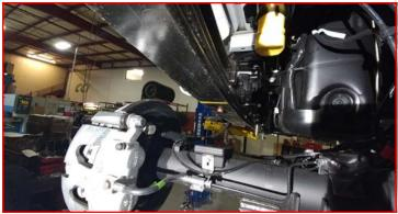
Locate the driver side lift block (Has a D cut into it under the bump stop tang). Raise the axle and the block up to the spring while aligning the center pin. (If tapered, make sure small end points to the front of the vehicle.) Install the provided u-bolts, and nuts. Snug the u-bolt nuts but do not fully tighten at this time. Repeat steps for passenger side.
