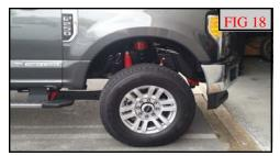
Jounce the suspension a few times to settle to the new ride height. Torque the radius arm brackets and arm bolts to 200 ftlbs, and track bar to 250 ft-lbs.
