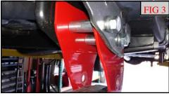
Remove the radius arm from the frame. Rotate the axle until there is enough clearance to install the ReadyLIFT® radius arm drop brackets. (Fig 2)
