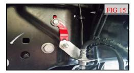
Remove the factory bump stop by pulling it out of its mount. Remove the mount from the frame. (Fig 16)
