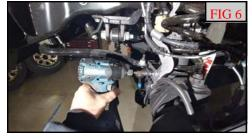
Remove the brake line bracket at the frame and axle. (Fig 5, 6)
