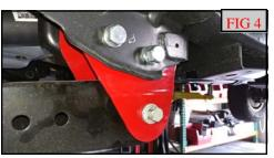
Install the ReadyLIFT® radius arm drop brackets into the frame using M18 x 130mm bolts, washers, crush sleeve, and nuts. Do not tighten at this time. (Fig 3)
