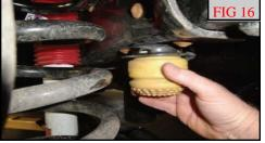
Install the bump stop to the factory mount by pressing it back into place. (Fig 17)
