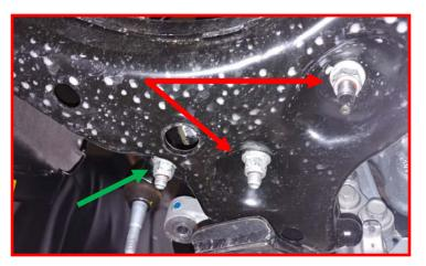
Carefully lower the control arm and knuck-le assembly down until the strut clears the control arm. Make sure to not over extend the brake lines and ABS harness. Adjust as necessary. To aid in removal, push knuckle towards the frame as you lower the control arm. Remove the strut from the vehicle by undoing the upper strut hardware.
