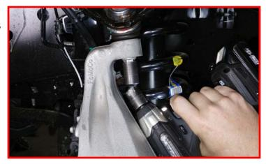
Loosen but do not remove the upper control arm hardware. Raise the upper control arm up and tilt the knuckle away from the frame. Carefully disengage the CV axle from the hub and actuator. Be careful not to damage the Vacuum actuator. The internals are made of plastic and easily damaged.
