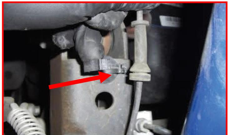
Remove the ABS wire clip at the frame rail. Let the ABS wire hang out of the way.
