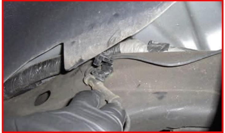
Remove the brake line bracket on the differential.
