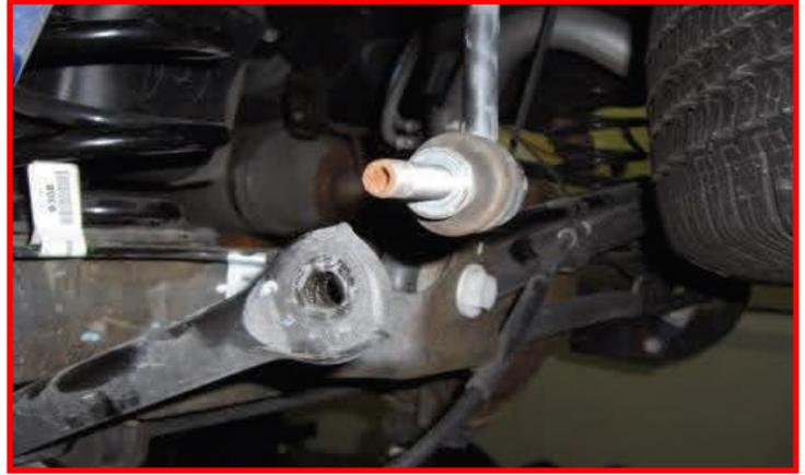
Reconnect the lower shock using the **factory hardware**. Do not tighten at this time.
