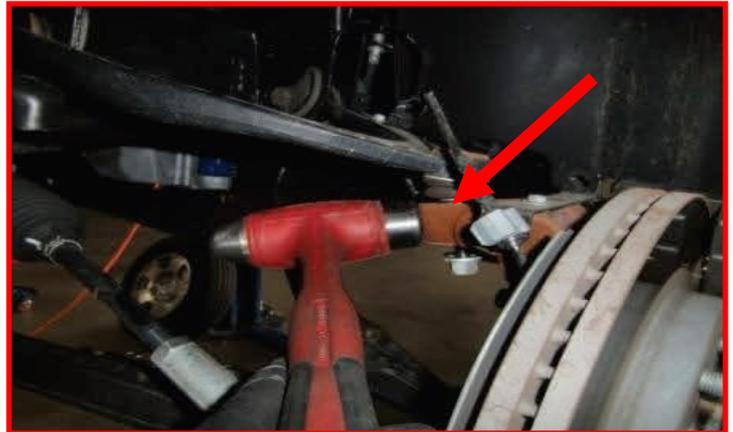
Support the lower control arm with a suitable jack, remove the lower strut hardware. Loosen but do not remove the lower control arm hardware at the frame.
