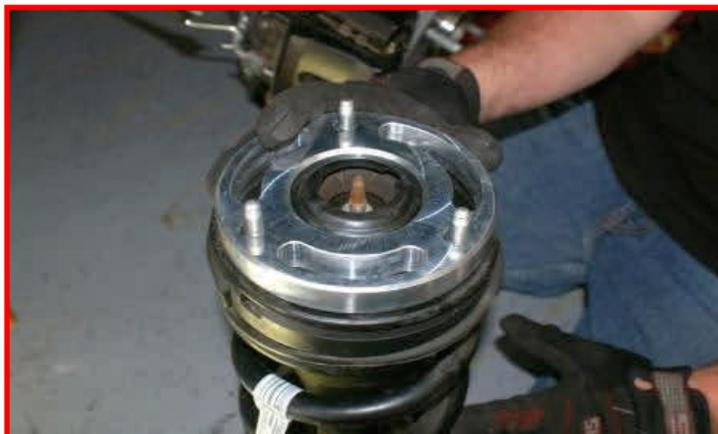
Install the strut assembly into the vehicle using the provided **M10 flange nuts**. Do not tighten at this time.
