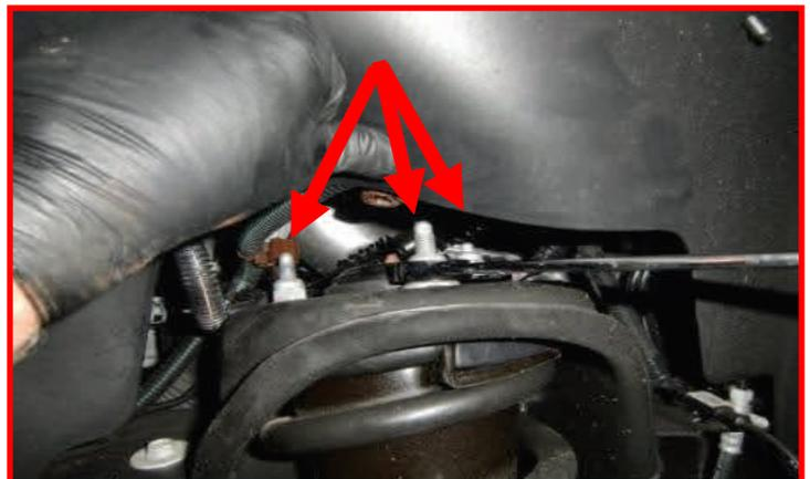
Place the ReadyLIFT upper strut extension to the top of the strut.
