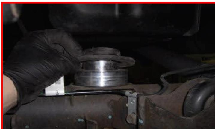
Install the springs back into the vehicle. Raise the axle up to hold the springs in place.
