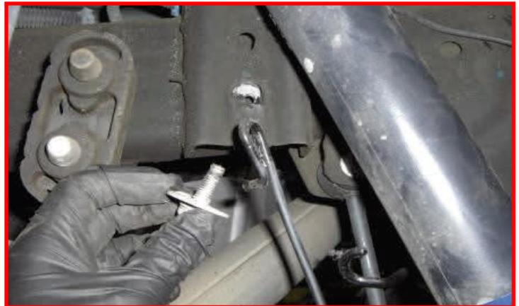
Support the axle with a suitable jack. Remove the lower shock mount from the axle.
