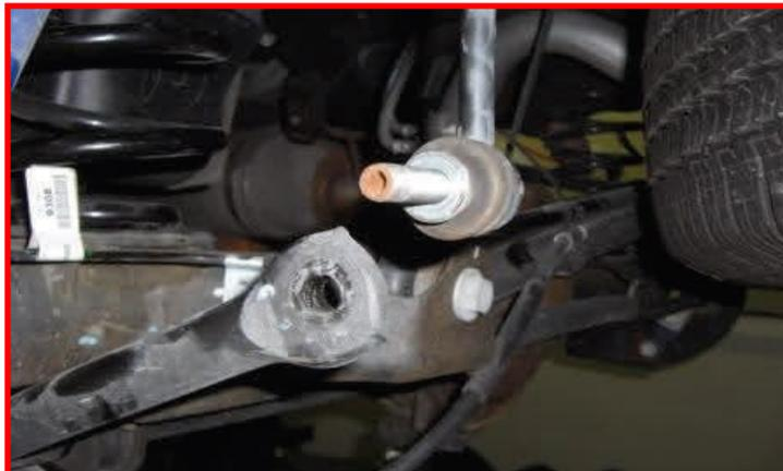
Carefully lower the axle down while keeping an eye on the brake lines and ABS wires. Remove the rear springs from the vehicle. Remove the rubber isolator from the axle.
