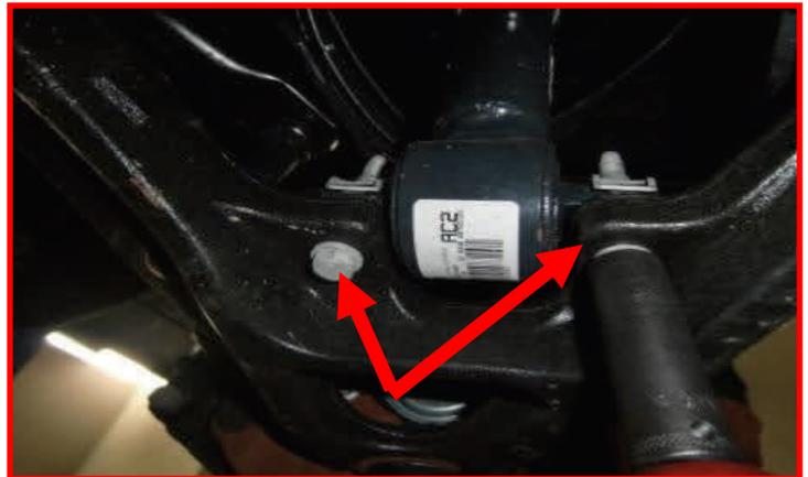
Remove all electrical harness clips on the top of the upper strut studs. Magna-ride vehicles disconnect the electrical connector attached to the strut. Remove the upper strut hardware. Remove the strut from the vehicle.
