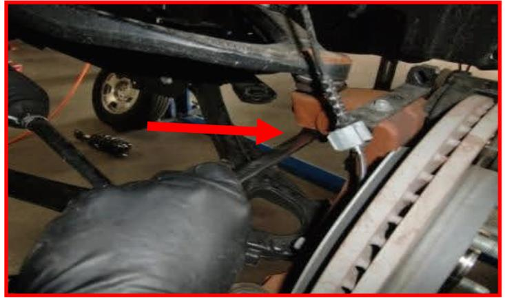
Strike the upper ball joint boss on the knuckle with a dead blow hammer to dislodge the taper. Disconnect the upper ball joint completely and let the knuckle hang out of the way. Make sure to not over extend the brake/ABS lines. Adjust as necessary.
