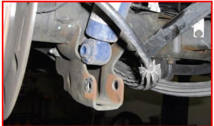
Remove the lower sway bar end link from the sway bar. Let hang out of the way.
