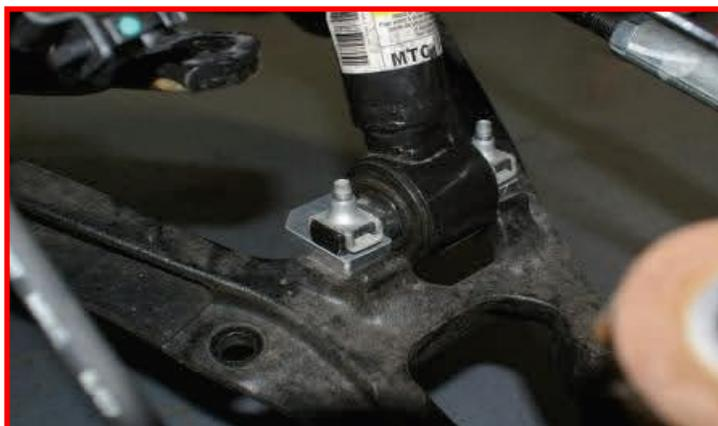
Install the upper ball joint to the knuckle using the **factory hardware**. Torque to **65 ft-lbs**.
