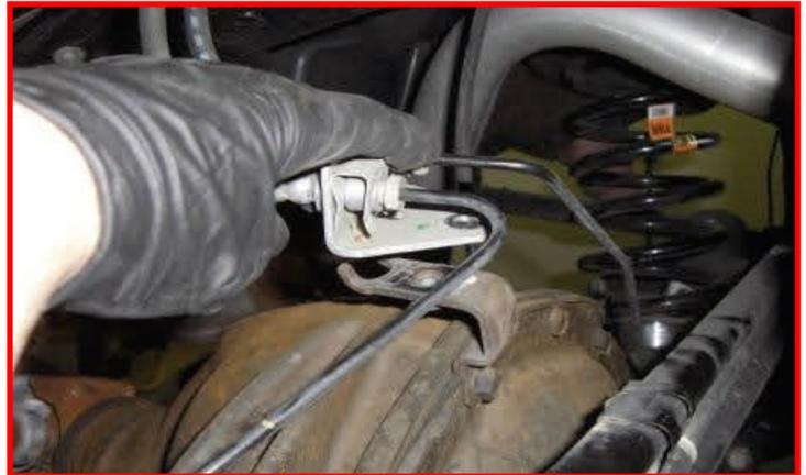
Remove the parking brake bracket on the frame rail. Let hang out of the way.
