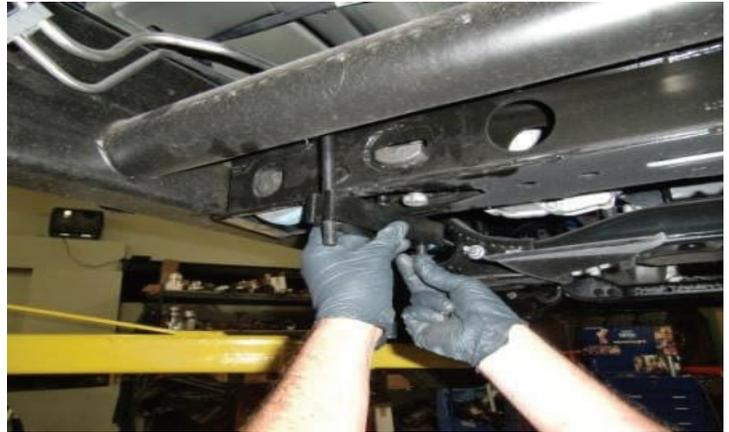
Once the keyway is adjusted high enough, remove the cross pin. **DO NOT push it through with your finger.** Always pull it out away from the keyway. Once the cross pin is out, remove the torsion bar unloading tool.
