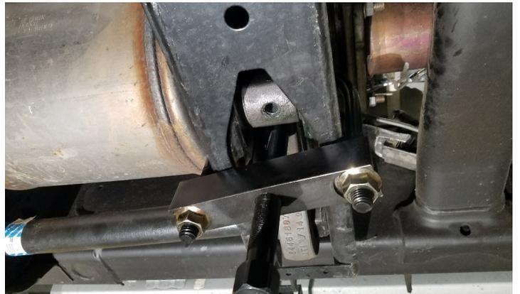
Standard model torsion bar reuse factory torsion arm adjustment bolt.
