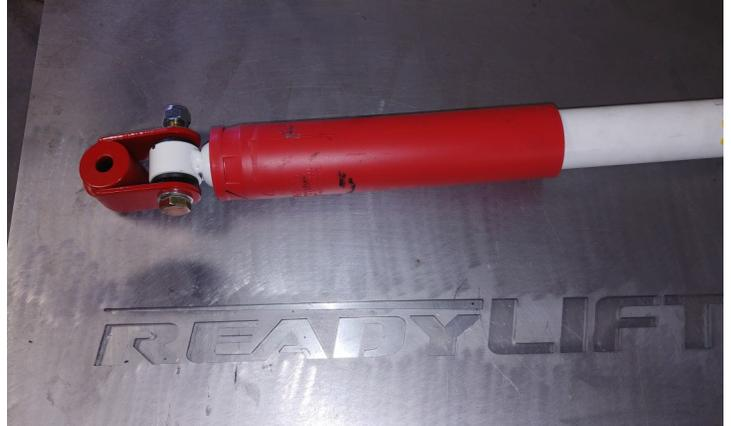
Reattach the shock to the frame using factory hardware. Hand tighten only, final torque will be done when the vehicle is on the ground.
