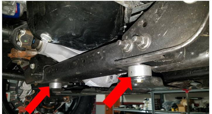
Trim the plastic gravel guard. **Cut a slot just large enough for a 3/8 bolt to slide freely**, on the lower mount that connects the gravel guard to the skid plate. **Use the provided spacers large washers and bolts to attach at the lower mount.** Hand tighten only. **Use the factory hardware** to attach the top of the gravel guard in its original position. Torque all bolts to 25ft-lbs.
