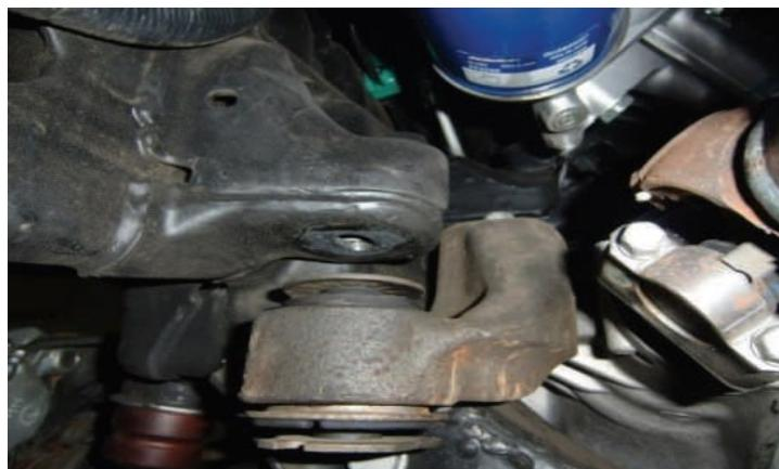
Install the ReadyLIFT **differential spacers** between the differential cradle and frame using the provided **bolts and laser cut washers**. Use factory flange nuts. Torque all to **95 ft-lbs**.
