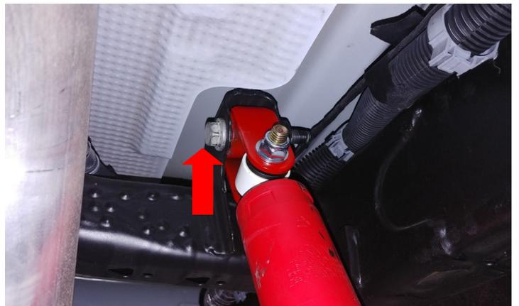
Reattach the shock to the axle using factory hardware. Hand tighten only, final torque will be done when the vehicle is on the ground.
