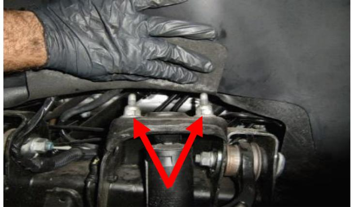
Add shock spacer to the upper mounting studs. Reinstall the shock to the upper mount. Use provided hardware torque to 45ft-lbs.
