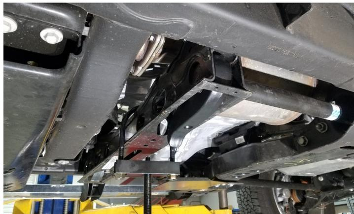
**The included differential and skid plate spacers are optional but recommended to minimize drivetrain noise and/or prevent premature wear on the CV axles and drivetrain.**
