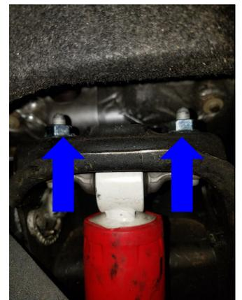
Measure and record the torsion key adjustment bolt length and part number. Remove the torsion bar adjustment bolt.
