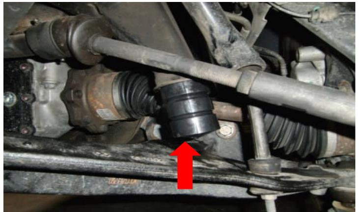
Use the torsion bar unloading tool, load the torsion bar enough to install the cross pin. **DO NOT pull it through with your fingers.**
