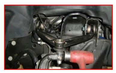
Remove the upper control arm bolts from the frame rails. Mark the cam bolt and cam orientation for re-installation.
