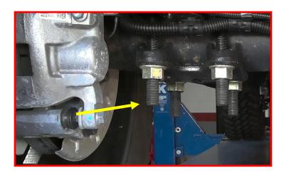
Install the Falcon rear shocks using the factory hardware.
