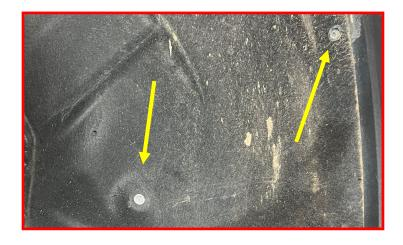
Remove the outer most rear tab on the factory mud flap.
