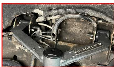
Install the upper control arm ball joint to the factory knuckle using the provided hardware.
