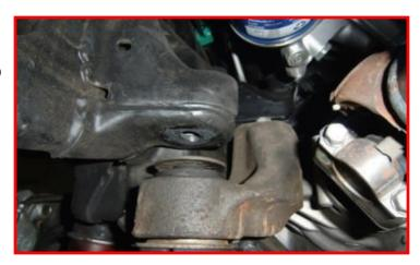
Install the 1/2" ReadyLIFT differential spacers between the frame and differential cradle. Use the provided laser cut washers and M14x130 bolts, reuse factory flange nuts.
