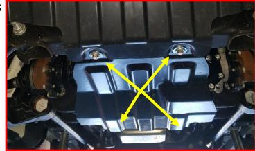
Locate the four (4) front and rear differential cradle bolts. Remove all four and lower the differential down enough to install the 1/2" differential spacers.
