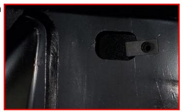
Attach the fender liner using the 1/4 fender washer and thread cutting bolt.
