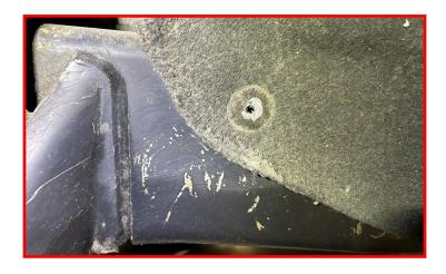
Install the provided U-nut to the frame (on vehicles with slot).
