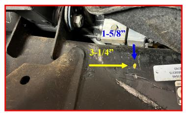
Debur the hole and coat with some type of anti-corrosion coating such as undercoating or paint.
