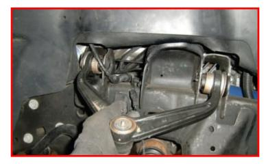
Install the ReadyLIFT upper control arm to the frame using the factory cam bolts and cams.
