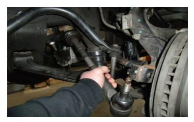
Install the outer tie rod end to the knuckle using the provided hardware. Torque to 65 ft-lbs.
