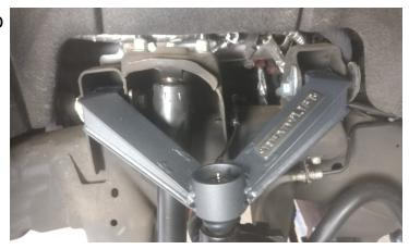
Install the upper control arm ball joint to the factory knuckle using the provided hardware. Torque to 85 ft-lbs. Grease the upper ball joint using a high quality ball joint grease. DO NOT over grease. Install the ReadyLIFT ball joint cover (shown) by pressing into place.
