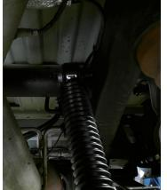
Reattach the brake line bracket to the axle. Use factory hardware torque to 5ft-lbs.
