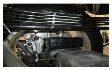
Raise the axle with the ReadyLIFT block installed to the leaf pack. Install the provided U-bolts and hardware. Only snug the U-bolts up enough to hold the axle in place. Repeat all steps on the passenger side. Final torque will be done when the vehicle is on the ground. Repeat the block installation on the passenger side.
