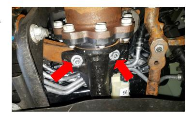
On the passenger side add two of the 68-3035CDS spacer between the frame cradle and the differential. Use provided hardware Torque to 65 ft-lbs.
