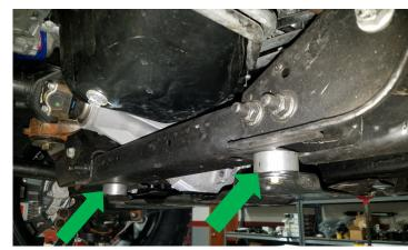
The lower mount of gravel guard must be trimmed. Cut a slot large enough for the provided M10 bolt to slide freely. Use the provided M10x45 bolts, M10 fender washer, and 7/8" spacers to attach the skid plate and gravel guard. Hand tighten only. Use the factory hardware to attach the top of the gravel guard in its original position. Torque all skid plate and gravel guard bolts to 25ft-lbs.
