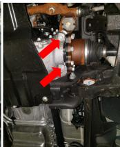
On the driver side add three of the 68-3035CDS spacer between the frame cradle and the differential. Use factory hardware hand tighten at this time.
