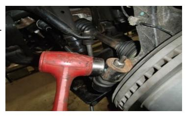
Use the appropriate tool, rotate the inner tie rod counter clock wise to remove the tie rod from the center link. Discard the factory tie rod.
