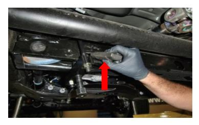
Push the torsion bar forward through the factory keyway cross member and lower control arm. You may need to use a hammer and punch on the end of the bar to break it loose from the keyway and control arm.
