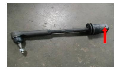
Use a drop of thread locker on the threaded end of the supplied tie rod. Install the supplied tie rod assembly to the center link. Fully tighten the inner tie rod to the center link.
