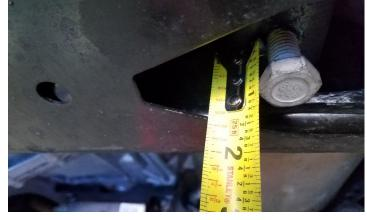
Using a torsion bar unloading tool (ReadyLIFT part #66-7816A), relieve the pressure on the torsion key cross pin. CAUTION: Take care as the torsion key is under extreme pressure and can cause injury and/or death if handled improperly. Always use safety equipment.
