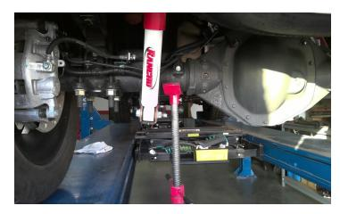
Loosen but do not remove the U-bolts on the passenger side. Remove the U-bolts completely from the driver side. Discard the factory U-bolts, washers, and nuts.
