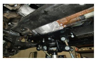
Locate the front and rear differential cradle bolts. Remove all and lower the differential down enough to install the differential spacers.
