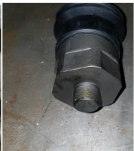
Locate the ReadyLIFT tie rod assembly. Install the provided Zerk fittings into the inner and outer tie rod end. There are 2 for the inner.
