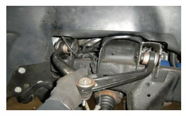
Install the ReadyLIFT upper control arm to the frame using the factory cam bolts and cams. Torque to 125 ft-lbs.
