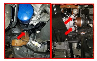
On the driver side add three of the 68-3035CDS spacer between the frame cradle and the differential. Use factory hardware hand tighten at this time.
