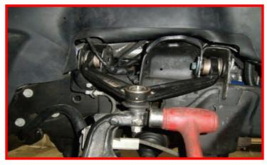
Remove the upper control arm from the frame rails. Mark the cam bolt and cam orientation for re-installation.
