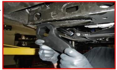
Remove the front skid plate from the cross members. Loosen the but do not remove the lower control arm hardware.
