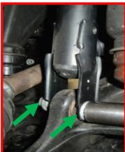
Install the Falcon front shock using the hardware pack supplied with the shocks for the upper mount and the factory hardware for the lower mount.
