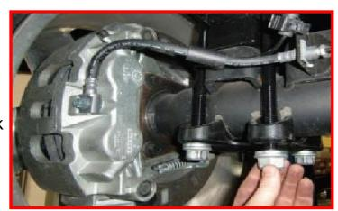
Install the Bilstein shocks to the frame using factory hardware. Hand tighten only, final torque will be done when the vehicle is on the ground.
