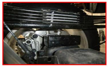
Raise the axle with the ReadyLIFT block installed to the leaf pack. Install the provided U-bolts and hardware. Only snug the U-bolts up enough to hold the axle in place. Repeat all steps on the passenger side. Final torque will be done when the vehicle is on the ground. Repeat the block installation on the passenger side.
