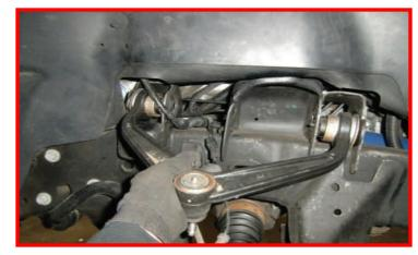
Install the provided clip nut through the factory droop limiter.
