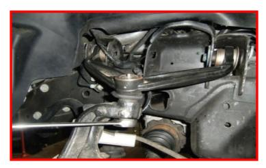
Strike the ball joint boss with a dead blow hammer to dislodge the taper.
