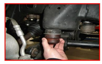
Install the ReadyLIFT bump stops. Use a soapy water solution to aid in install. You may need to use the lower control arm and a jack to "press" them into place.
