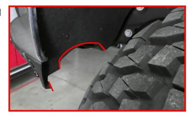
For negative offset wheels you may need to trim the plastic mud flap on the back side of the wheel. Trim the front side of the mud flap only.
