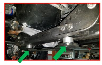
The lower mount of gravel guard must be trimmed. Cut a slot large enough for the provided M10 bolt to slide freely. Use the provided M10x45 bolts, M10 fender washer, and 7/8" spacers to attach the skid plate and gravel guard. Hand tighten only. Use the factory hardware to attach the top of the gravel guard in its original position. Torque all skid plate and gravel guard bolts to 25ft-lbs.
