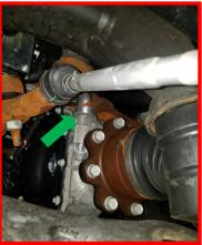
Locate and remove the two passenger side flange nuts that mount the differential to the frame cradle. Discard factory hardware.
