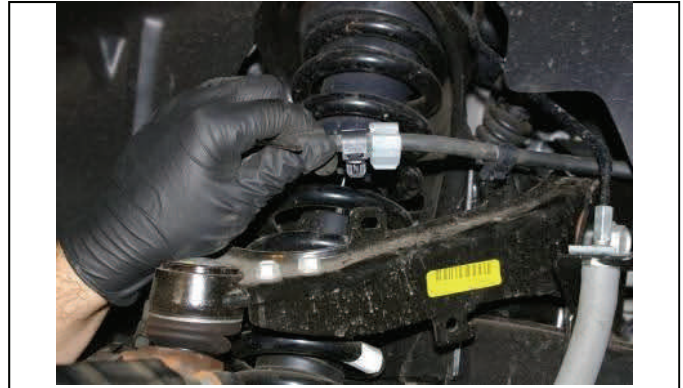
Unclip brake lines from upper control arms
