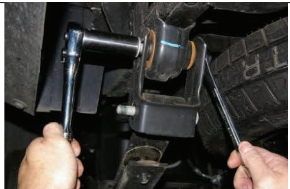
Disconnect and remove shackles
