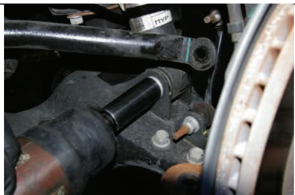
Remove lower strut mounting hardware
