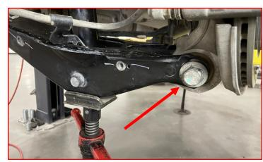
Install the brake line brackets to the lower control arm.
