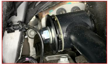
Once upper control arms have been properly torqued, install completed strut assembly. Install with supplied M10 nuts.
