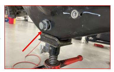
Measure the strut studs to 1.25" from the top of the strut. Use an appropriate cutting tool to trim studs to the measured height.
