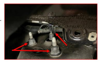
Remove the lower knuckle bolt. Lower the jack enough to allow for the knuckle to release from the lower control arm.
