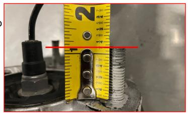
Install strut top spacer onto strut assembly. Using the factory nuts, install, tighten and torque nuts to 35-ft/lbs.
