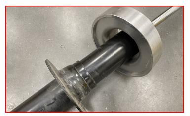
Using the ReadyLift Rear Strut Spacer as a guide, align the strut so the lower strut bolt hole is perpendicular to the two studs in the Rear Strut Spacer.
