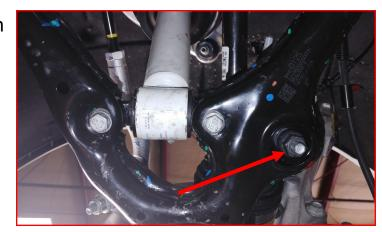
Remove the axle nut. Press axle back through hub to allow for greater misalignment and ease in the removal/instillation process.
