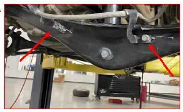
Install the two (2) fender liner screws.
