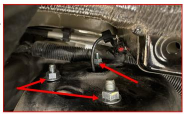
Install but do not tighten the lower strut bolt.
