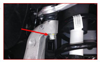
Support the lower control arm with a suitable jack. Remove the lower strut mounting bolt from the lower control arm. Discard factory bolts.
