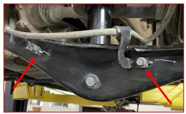
Support the lower control arm with a suitable jack. Peal back the fender liner to remove the three (3) upper strut bolts.
