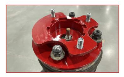
Using the supplied M10-1.25 Serrated Flange nuts, install the rear strut assembly into the strut tower.
