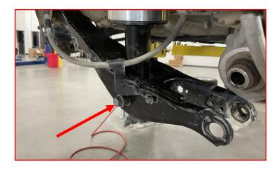
Using a suitable jack, raise the lower control arm enough to install the lower knuckle bolt.
