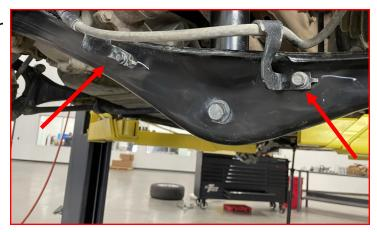
Install the two (2) fender liner screws.
