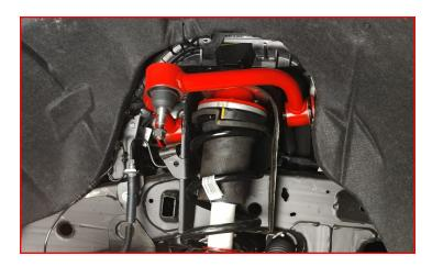
Remove the lower nut clip from the strut and discard.
