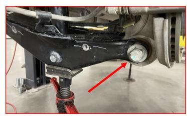
Install the brake line brackets to the lower control arm.
