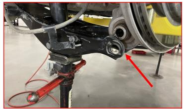
Remove the strut nut and bolt. Retain factory hardware.
