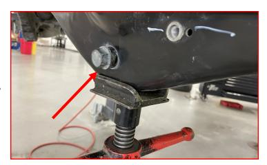
Measure the strut studs to 1.25" from the top of the strut. Use an appropriate cutting tool to trim studs to the measured height.
