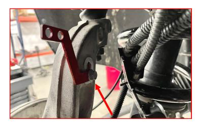
Install the factory harness bracket to the Magnetic Ride Relocation Bracket using the supplied M6 bolt, nut, and washers
