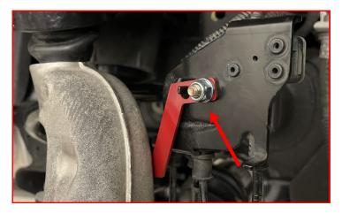
Remove the factory brake pad sensor bracket from the knuckle.
