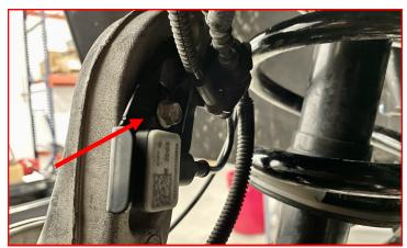
Install the Magnetic Ride Relocation Bracket to the backside of the knuckle using factory hardware.
