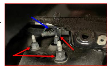
Remove the lower knuckle bolt. Lower the jack enough to allow for the knuckle to release from the lower control arm.
