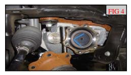
Carefully lower differential out of the vehicle and set aside for modifications.
