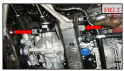
Remove the bolts holding the hangers to the frame. Lower the differential down until you can insert the ReadyLIFT® diff drops into place. The large spacers go in between the front side of the hanger and frame and the small spacers go in between the rear side of the hanger and frame. Install using M12 x 120mm bolts, washers and nuts. Torque to 50 ft-lbs. (Fig 3)
