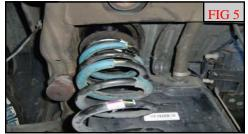
Install the coil springs with the factory isolators. Raise the axle enough to hold them in place. (Fig 5)
