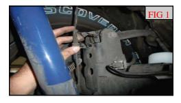
Remove the ABS and brake line at the frame and axle to gain slack to work. (Fig 1)
