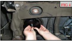
Install the ReadyLIFT® spring spacer using the ReadyLIFT® nut plate on top of the frame, M12 bolts, lock washer and flat washers. Torque to 50 ft-lbs. (Fig 3, 4)
