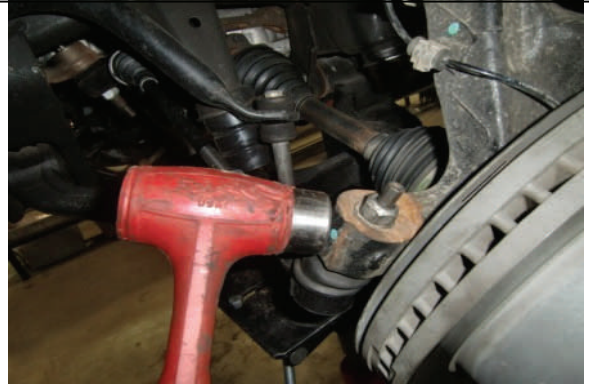
Disconnect outer tie rod nut and strike spindle to disconnect.
