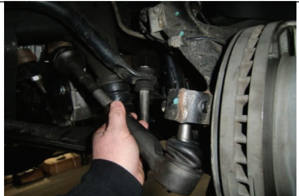
Attach outer tie rod to spindle and tighten
