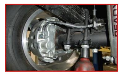
Lower the axle down enough to install the ReadyLIFT block. Make sure that if the block is tapered, to install the small end of the block towards the front of the vehicle.
