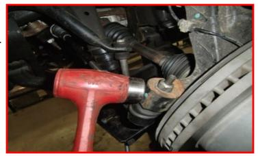
Remove the inner tie rod from the center link. Discard both inner and outer tie rod ends as they will not be reused.
