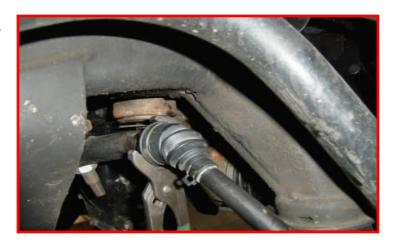
Locate the ReadyLIFT tie rod assembly. Install the provided zerk fittings into the inner and outer tie rod end. There are 2 for the inner.
