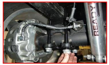
Install the ReadyLIFT provided shocks using the factory hardware. Do not tighten at this time. Make sure to install the SST3000 shock with the black body to the axle. Upgraded inverted shock shown in the picture. Install the rear wheels and lower the vehicle to the ground. Torque the lug nuts to the wheel manufacturer's specs. Jounce the vehicle to settle it to the new ride height.
