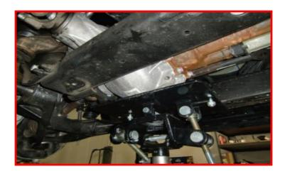
Locate the front and rear differential hanger bolts. Remove all and lower the differential down enough to install the differential spacers.
