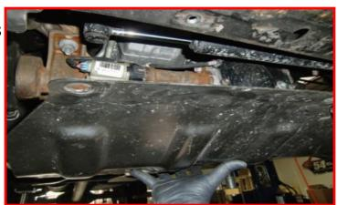
Loosen but do not remove the outer tie rod end nut at the knuckle. Strike the tie rod boss with a dead blow hammer to dislodge the taper. Remove the tie rod after this has been completed.
