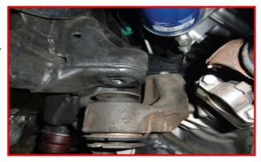
Install the ReadyLIFT differential spacers between the differential hanger and frame using the provided hardware. Torque all to 95 ft-lbs. Make sure that both horseshoe mounts clear the control arm pockets. It may be necessary to grind some material off the mounts to gain clearance.
