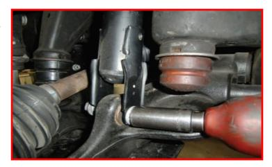
Remove the torsion bar adjustment bolt.
