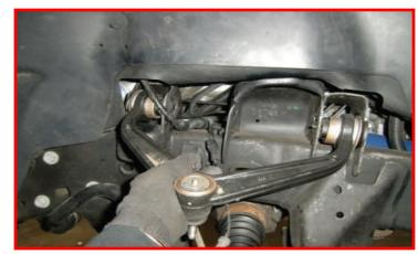
Install the clip nut into the droop limit pocket. Install the provided rubber droop limiter by screwing into the clip nut.
