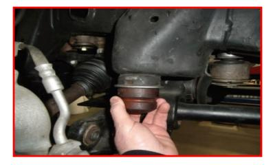
Install the ReadyLIFT bump stops. Use a soapy water solution to aid in install. You may need to use the lower control arm and a jack to "press" them into place. Install the ReadyLIFT front shock using the factory hardware. Do not tighten at this time.
