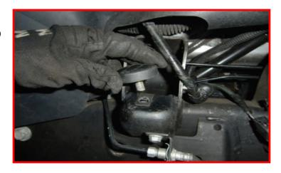
Install the ReadyLIFT upper control arm to the frame using the factory cam bolts and cams. Torque to 125 ft-lbs. Install the upper control arm ball joint to the factory knuckle using the provided hardware. Torque to 85 ft-lbs. Grease the upper ball joint using a high quality ball joint grease. DO NOT over grease.
