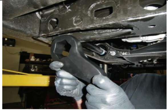
Install new torsion key and slide bar into position
