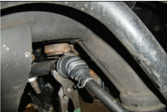
Loosen and remove inner/outer tie rod from center link.
