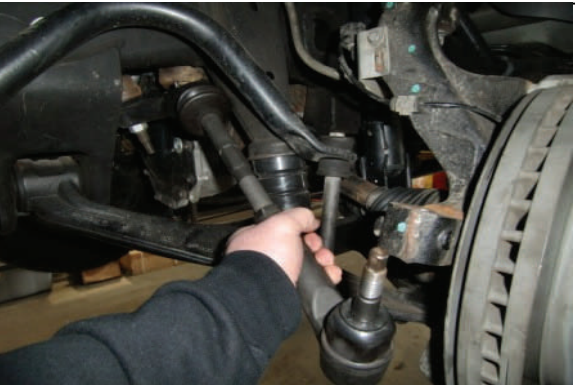
Install new steering assembly on center link
