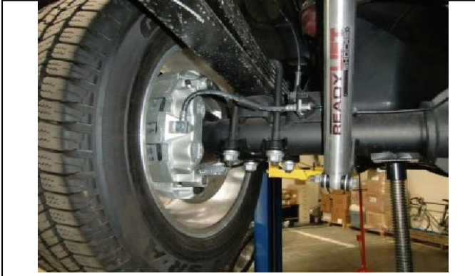
Properly support rear axle and disconnect lower shock mount
