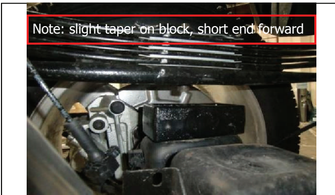
Locate lift block on axle mount and raise to meet leaf spring
