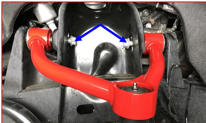
Install the completed strut assembly into the frame using **M10 flange nuts**.
