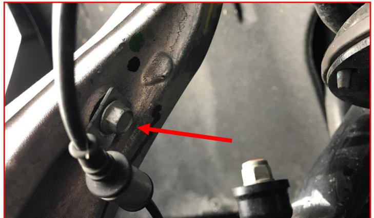
Remove the brake line bracket from the frame. Be sure to retain the **factory hardware**.
