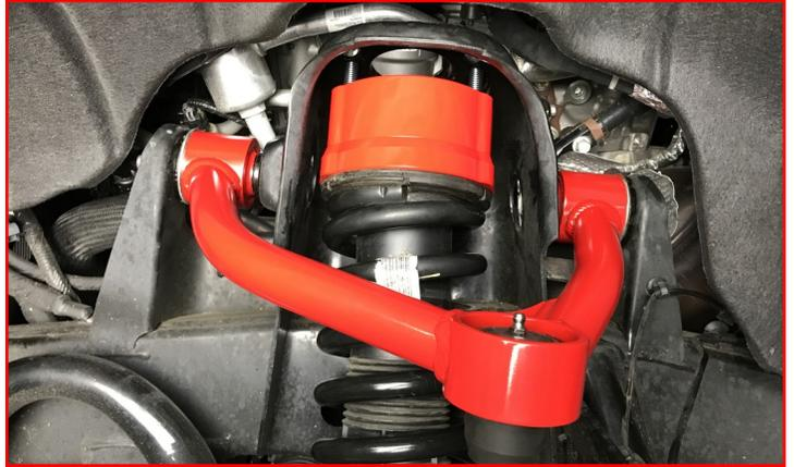
Raise the lower control arm up and install the lower strut mount using **factory hardware**. Do not tighten at this time.
