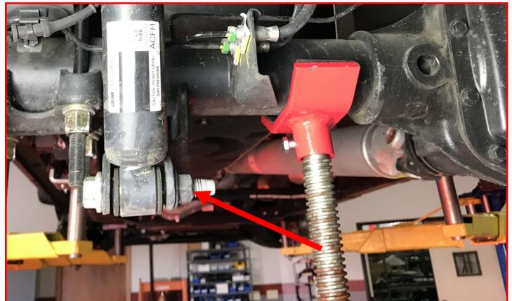
Loosen but do not remove the u-bolts on the passenger side. Completely remove the u-bolts on the driver side and discard. Lower the axle enough to install the ReadyLIFT block. Raise the axle while lining up the center pins on the axle and block. Install the provided u-bolts. Do not fully tighten at this time. Repeat for the other side of the vehicle.
