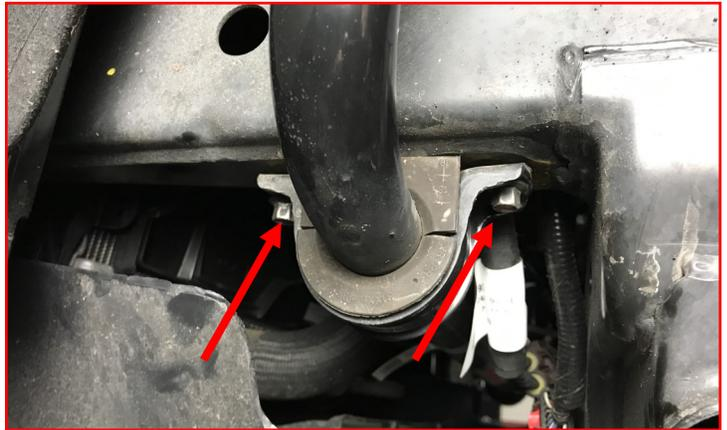
Install the sway bar drops to the frame using **factory hardware**. Torque to **45 ft-lbs**. Install the sway bar to the drop brackets using **M10 bolts, washers and M10 nuts**. Torque to **45 ft-lbs**.
