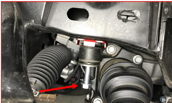
Release support from differential allowing the diff mounts to slide down mounting hardware. The differential may need a little assistance sliding down to the head of the bolt.
