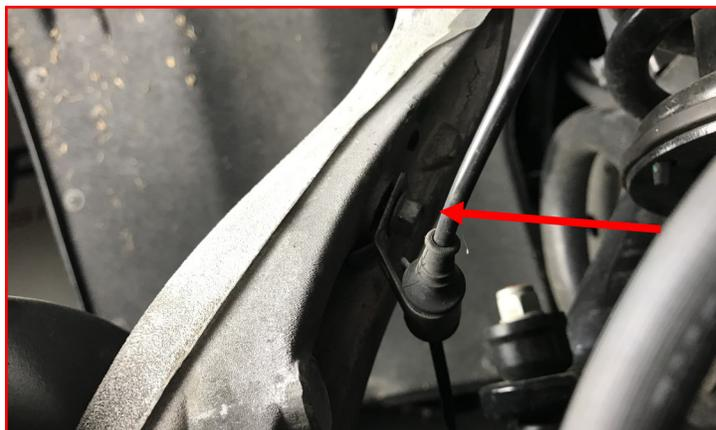
Install the front wheels and lower the vehicle to the ground. Jounce the suspension a few times to get it to settle to the new ride height. Torque the lug nuts to the wheel manufacturer specs, upper strut mount to **30-ft/lbs** and lower strut mount to **120-ft/lbs**. Torque lower control arm bolts, final torque will be set by alignment shop.
