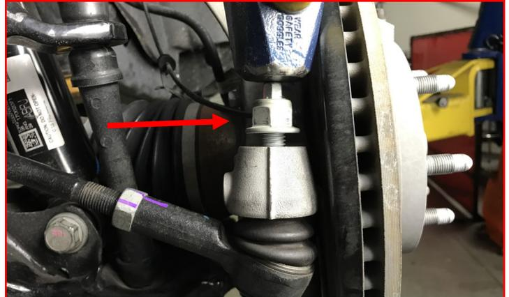
Remove the ABS sensor harness from the knuckle and hang out of the way.
