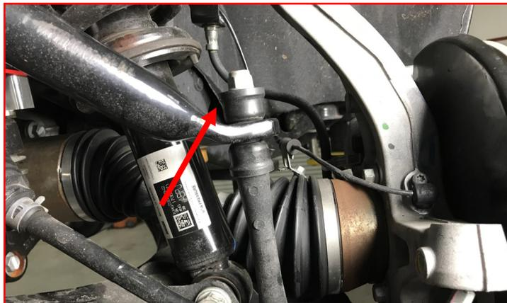
Loosen but do not remove **axle nut**. Press axle back through hub to allow for greater misalignment and ease in the removal/installation process.
