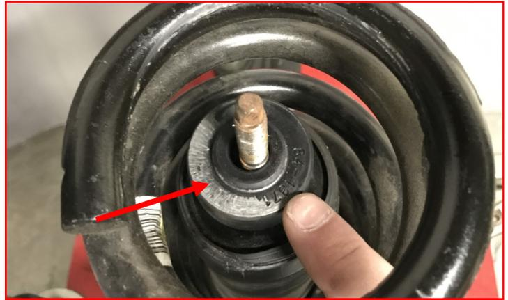
Install supplied **shock bushing crush sleeve** to shock shaft.
