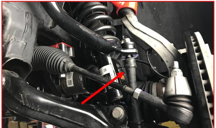
Install **brake line bracket spacer** using the factory hardware. Align bracket to match angle of the upper control arm and tighten.
