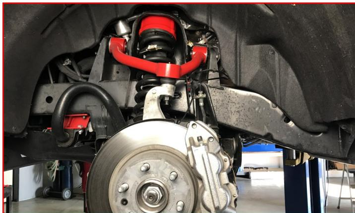
With the steering wheel centered, turn the tie rod ends until the tires are straight. If the steering wheel is not centered properly, the ABS/traction control lights may activate. Turn the wheels from lock to lock and make sure the brake lines and ABS routing clears all suspension components adequately. Reposition if necessary.
