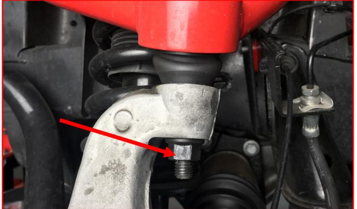
Install the **outer tie rod end** to the knuckle using factory hardware.
