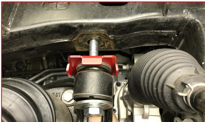
Install diff drop spacers between diff drop retainer and the differential mount.
