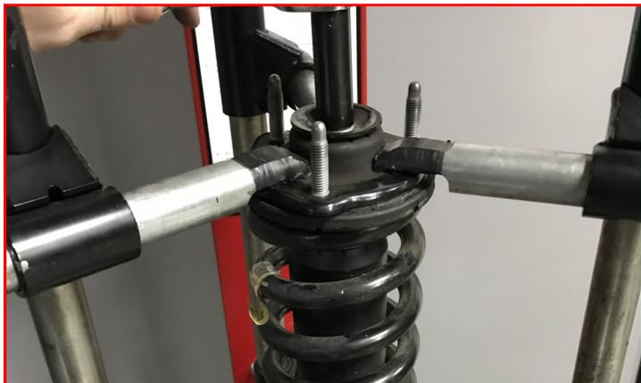
Install supplied **shock bushing half** to shock shaft.
