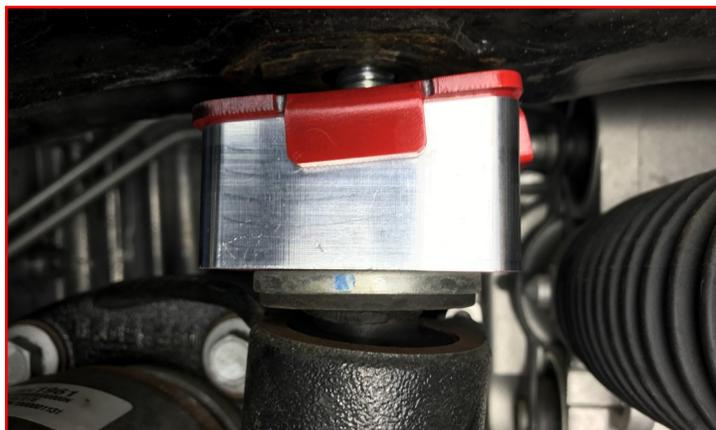
Tighten the differential bolts and torque to 100-ft./lbs.
