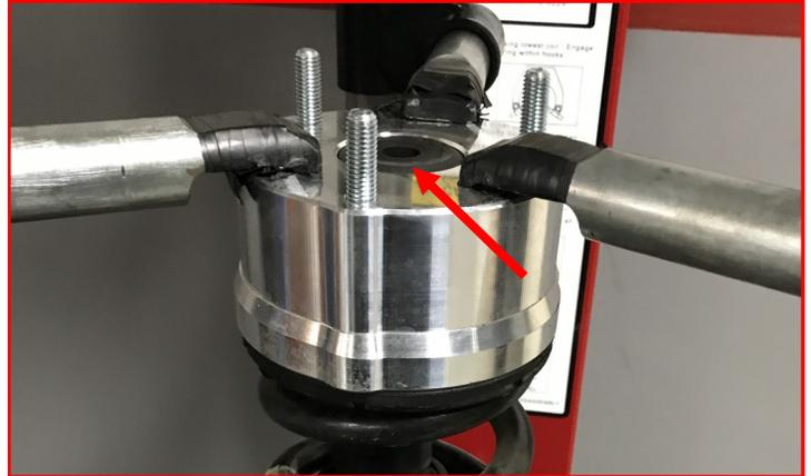
Install **factory washer** and supplied **M10 Flange nut** to shock shaft, tighten and torque to **30-ft./lbs.**
