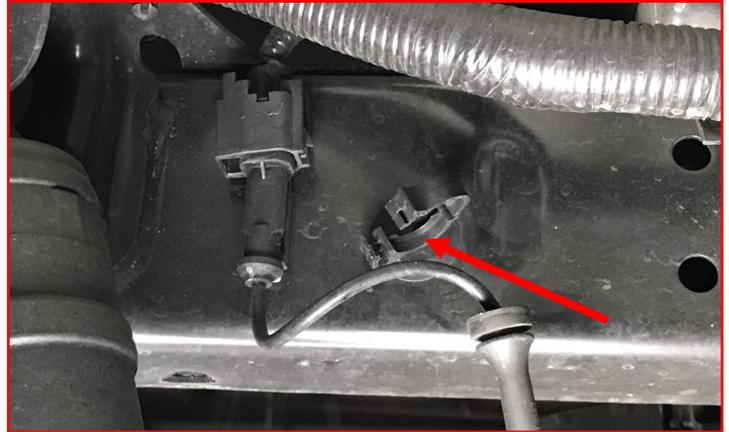
**Driver side:** Open the clip and remove the ABS wire.
