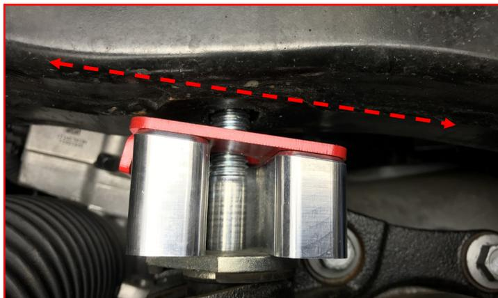
The diff drop retainer is designed to insure the diff drop will not dislodge under operating conditions. It is important the retainer ears are orientated so they contact the diff drop spacer on the three sides without the slot, effectively making the spacer solid.
