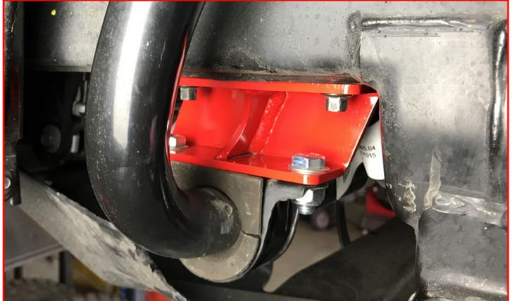
Install the **lower sway bar end link** to the control arm and sway bar. Torque to **35 ft-lbs**.
