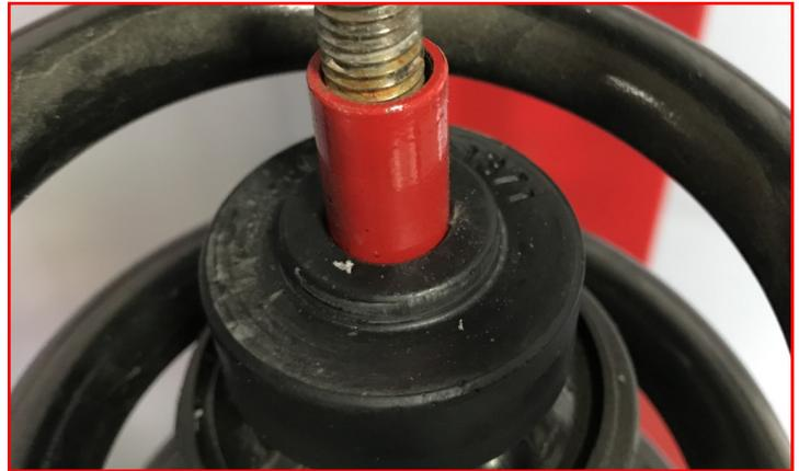
Install the replacement top hat and the rubber isolator taking care to install in same orientation as the factory top hat.
