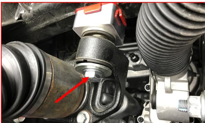
Install replacement upper control arm into frame pivot pockets using the factory hardware. Tighten hardware and torque to 85-ft./lbs.
