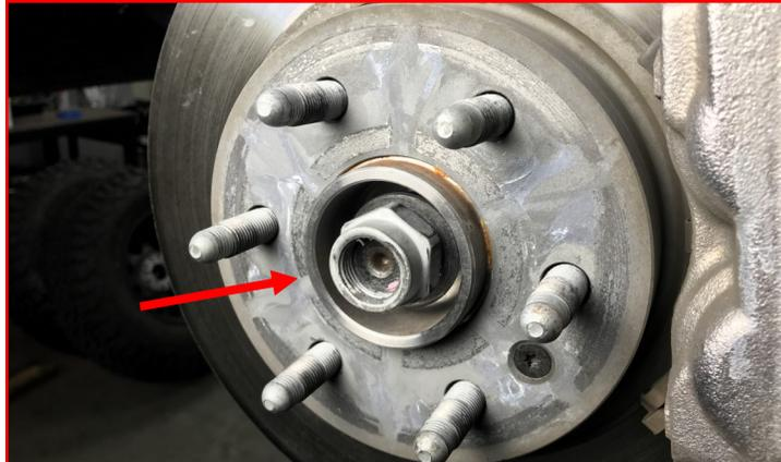
Remove the **upper control arm ball joint nut**. Strike the upper ball joint boss on knuckle with a dead blow hammer to dislodge the taper.
