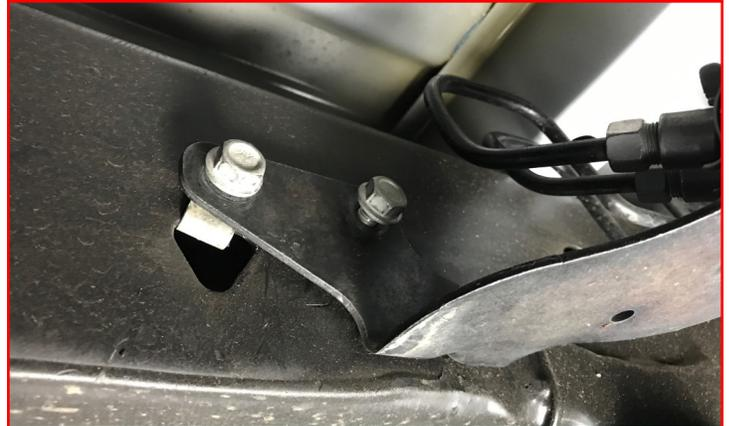
Install the rear wheels and lower vehicle to the ground. Torque the lug nuts to the wheel manufacturer specs, the U-bolts to **110 ft-lbs** and all shock hardware to **65 ft-lbs.**
