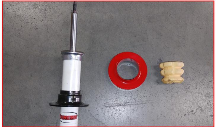
Ensure the orientation of the strut assembly is as factory, and install the shock. Using the spring compressor, compress the spring and install factory shock shaft nut.
