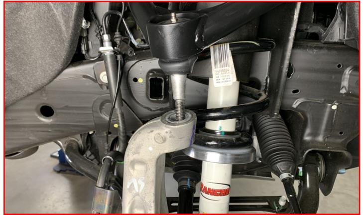
Install the **sway bar drop link** into the lower control arm using the factory nut.
