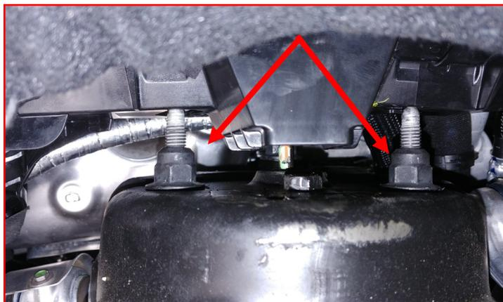
Remove the **upper control arm bolts** located inside the strut tower. Remove upper the control arm from the vehicle at this time. Discard the control arms.
