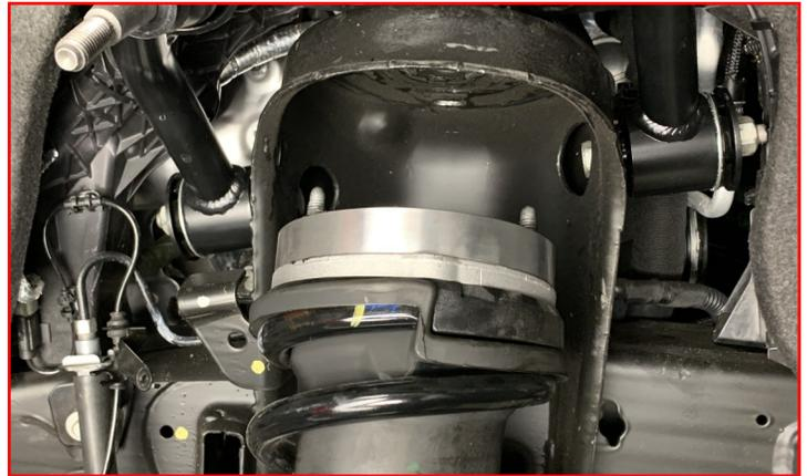
Install the factory lower strut bolts.
