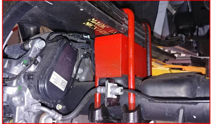
Install the lower shock to the axle using factory hardware. Do not tighten at this time.
