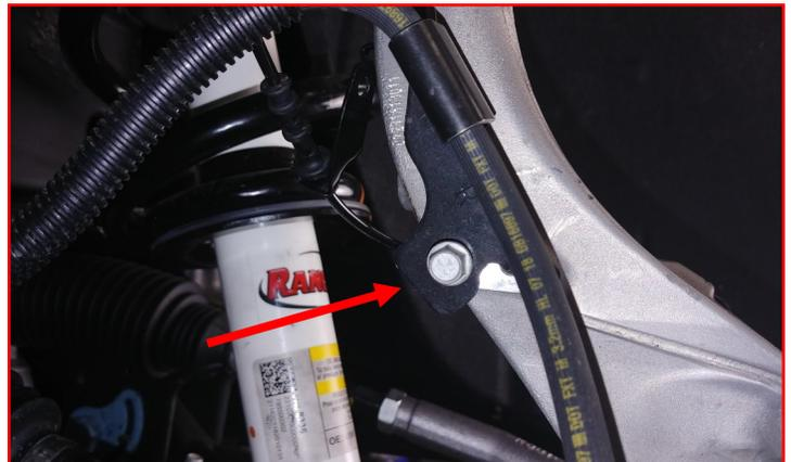
Remove the **ABS bracket** from the Upper Control Arm.
