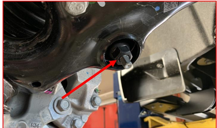
Install the **outer tie rod end** into the knuckle using the factory hardware.
