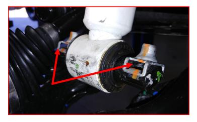
Install supplied M10 bolts through strut cross pin and lower control arm. Install M10 washers, and nuts on to bolts. Tighten and torque M10 nuts to 45-ft/lbs. Tighten upper strut nuts at this time. Torque nuts to 35-ft/lbs.
