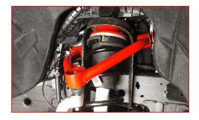
Insure the CV Axle is properly inserted and tighten axle nut. Torque to 160-ft/lbs.
