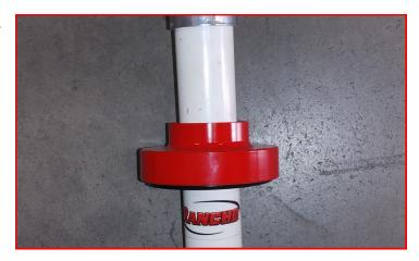
Insure orientation of the strut assembly is as factory, install the shock. Using the spring compressor, Compress spring and install factory shock nut. Tighten and torque to 30-ft/lbs.
