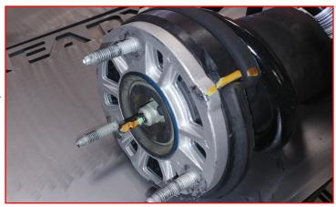
Using a spring compressor, relieve spring pressure from the strut top hat. Remove the factory top hat. Be sure to retain factory hardware.
