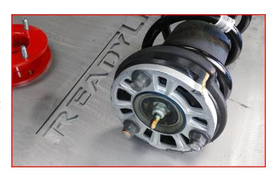
Install strut top spacer onto strut assembly. Using the supplied M10 nuts, install, tighten and torque nuts to 35-ft/lbs.
