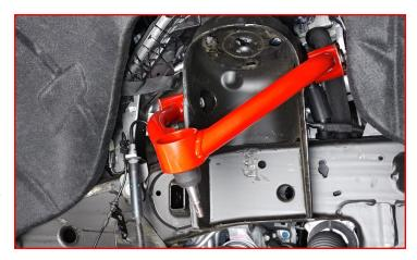
With the upper control arm bolts in place, install supplied laser cut washer and install, tighten and torque factory nuts to 90-ft/lbs.
