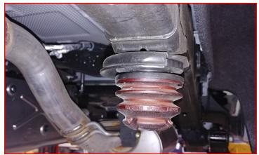
Install rear jounce stop extension between frame rail and jounce stop using supplied M10 Bolts and washers. Tighten and torque to 35 ft-lbs.
