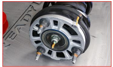
With studs marked, use appropriate cutting tool to trim studs to the proper height.
