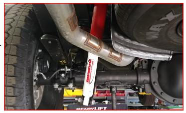
Remove the driver side u-bolts completely and discard. Lower the axle enough to remove the factory lift block making sure that all brake lines and ABS lines do not get over extended.
