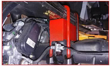
Install the shock extension using the provided M14 bolts, washers, and nuts to the top of the factory shock.
