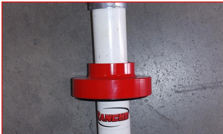
Ensure orientation of the strut assembly is as factory, install the shock. Using the spring compressor, Compress spring and install factory shock nut. Tighten and torque to **30-ft/lbs.**
