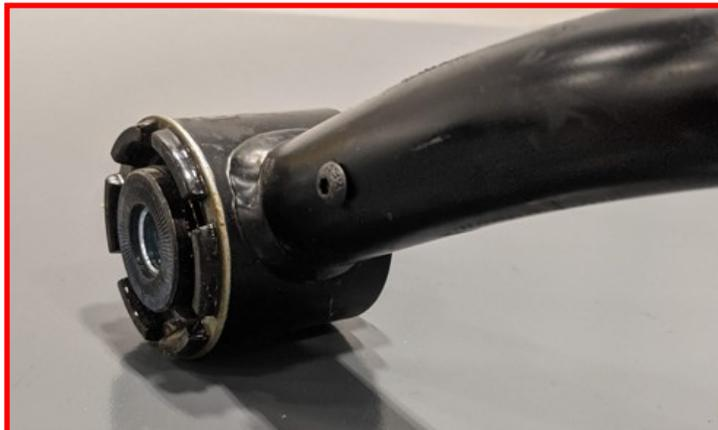
Install the ARC bracket on the on the arm using the provided button cap screw.
