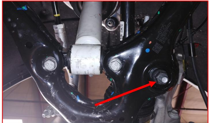
Remove the **axle nut**. Press axle back through hub to allow for greater misalignment and ease in the removal/installation process.
