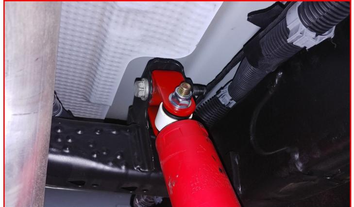
Remove factory bolt that attaches the rear bump stop to frame and discard the bolt.
