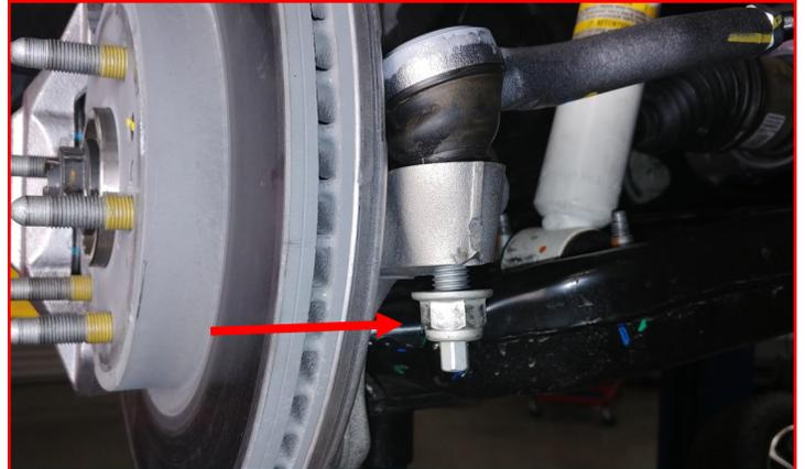
Remove the **ABS sensor harness and brake-line bracket** from the knuckle and hang out of the way.
