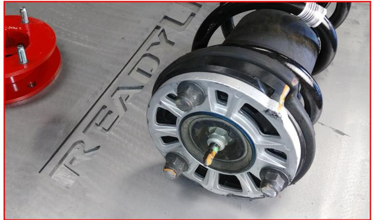
Install strut top spacer onto strut assembly. Using the supplied M10 nuts, install, tighten and torque nuts to 35-ft/lbs.
