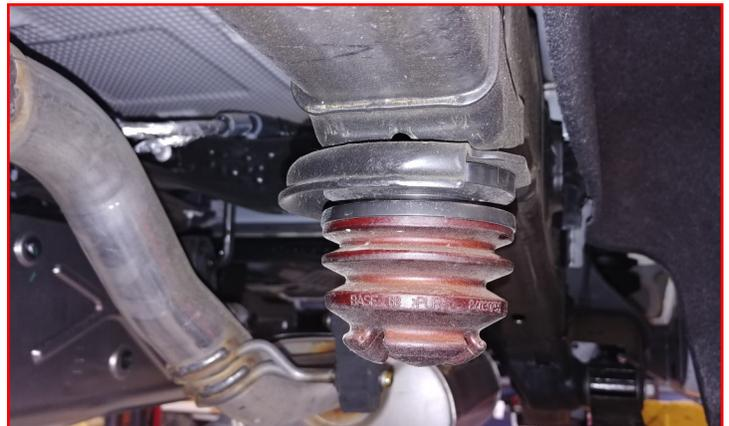
Install **rear bump stop extension** between frame rail and jounce stop using supplied M10 Bolts and washers. Tighten and torque to **35 ft-lbs.**
