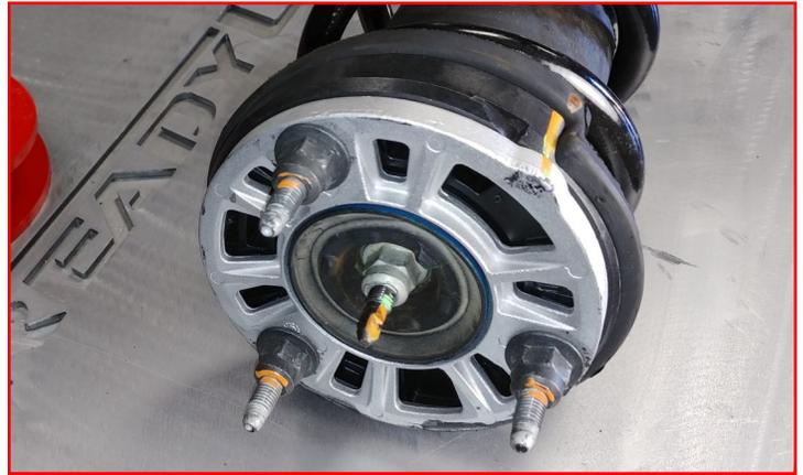
With studs marked, use appropriate cutting tool to trim studs to the proper height.
