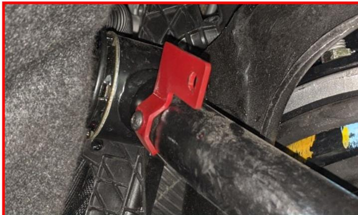
Insert the ball stud from the ARC sensor into the hole on the bracket. Use the provided 6mm nyloc nut to attach the ball stud to the bracket.
