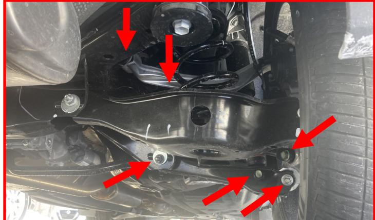
Once you've loosened the components on both sides of the vehicle, roll the vehicle back and forth a few times to let the suspension free itself.
