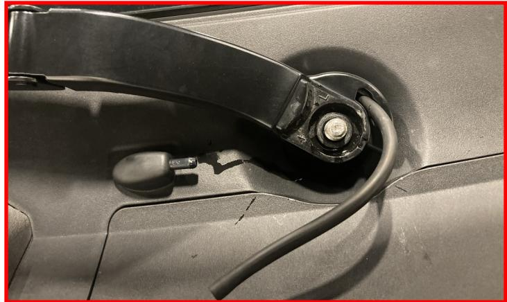
Remove the **factory molding clip** on the driver side connecting the molding to the wiper cowl.
