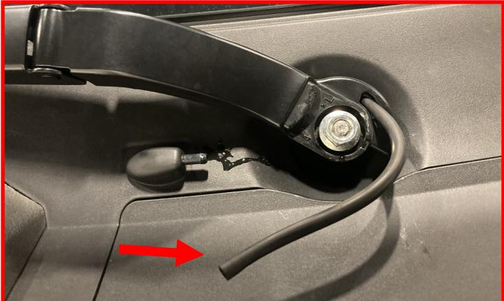
Remove the **factory mounting nut**. Mark the windshield wiper location against the shaft for reinstallation. Gently lift up on the wiper arm while slightly twisting. The arm should pop off the shaft.
