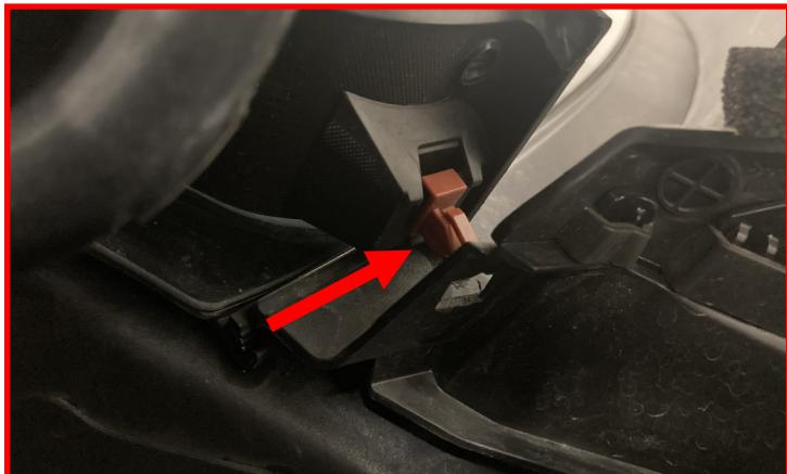
Re-install the **driver side molding clip** making sure that all the moldings are lined up before doing so.
