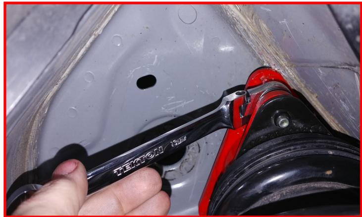
Raise suspension using the jack while lining the **upper strut extension** up with the bolt holes on the strut tower. Use of a helper will aid in the installation. Install the strut assembly to the strut tower using the **provided 3/8-16 bolts**.
