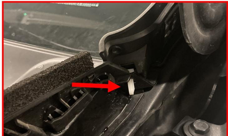
Remove the **factory molding clip** on the passenger side connecting the molding to the wiper cowl.
