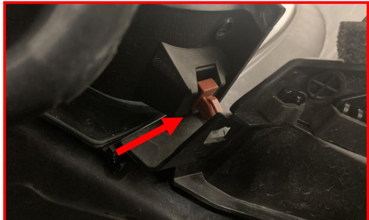
Locate the **x7 plastic clips** holding the cowl to the body. Remove all the clips and set aside. Gently lift up on cowling from the engine bay side, while lifting pull towards the front of the vehicle to disengage from the windshield. Once disengaged from the windshield, set aside in the engine bay.
