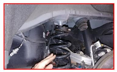
Install the ReadyLIFT rear spring spacer on top of the factory isolator. Install the spring back into the vehicle. Make sure the lower spring is orientated to the spring lock on the lower isolator.
