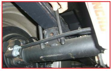
Disconnect the shock and remove it from the vehicle. Make sure you mark or take note of witch side is the top mounting side.
