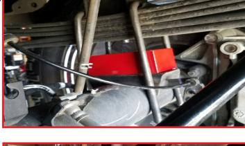
Raise the axle and reconnect the shock to the axle, using the factory hardware. Do not tighten at this time.
