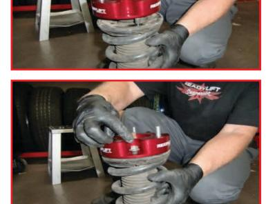
Raise the LCA, reconnect the strut to the lower control arm using the factory hardware. Do not tighten at this time.
