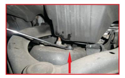
Disconnect driver and passenger side sway bar from the frame rails, and let hang out of the way.
