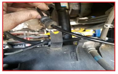
Remove the U bolt and hardware from the driver side only.
