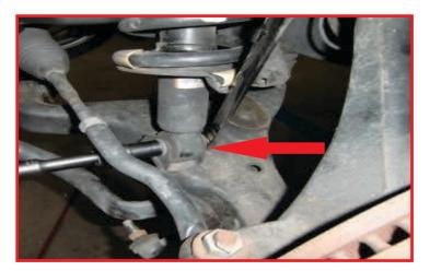
Reattach the upper ball joint to the knuckle using factory hardware. Torque to 65 ft-lbs.
