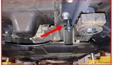
Install the front gravel guard to the core support cross member using the factory hardware. Do not tighten at this time.
