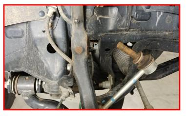
Remove the lower strut hardware.
