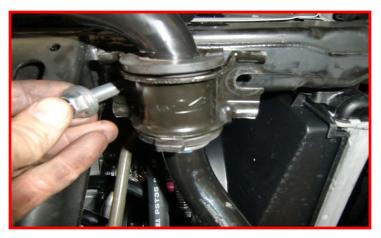
Install the ReadyLIFT sway bar brackets to the frame using the factory hardware. Torque to 35 ft-lbs.
