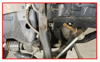
Remove the sway bar from the frame rail. Let hang out of the way.
