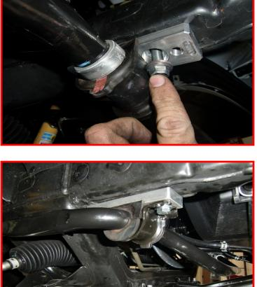
Install the sway bar to the ReadyLIFT brackets using the provided hardware. Torque to 35 ft-lbs.
