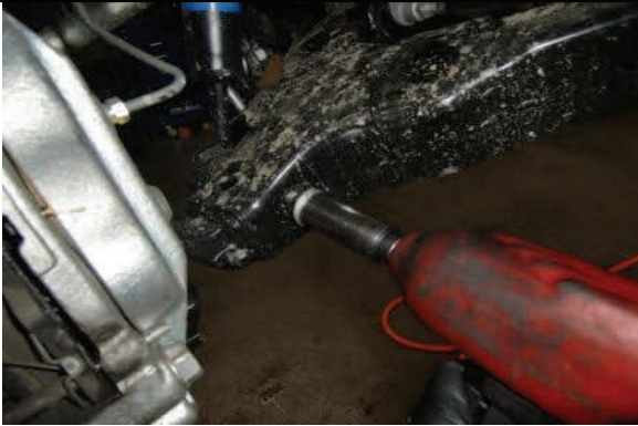
Reattach and tighten lower strut mounting hardware
