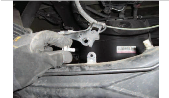
Disconnect ABS wiring brackets from axle.
