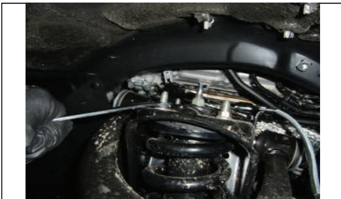
Remove upper strut mounting hardware
