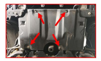
If equipped, remove the differential gravel guard.
