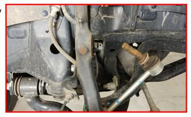
Remove the lower strut hardware.
