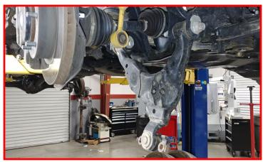
Remove the strut from the vehicle.
