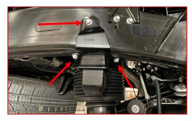
Using the supplied M8-1.25 x 40 hex head flange bolt and the aluminum crush sleeve, attach the bump stop extension to the frame using the top hole on the extension.
