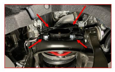
Tighten inner control arm hardware. Final torque spec must be set by alignment technician.
