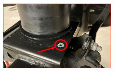
Seal the hole with an adequate coating.
