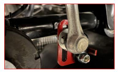
Remove the lower factory strut bushing from the shock.
