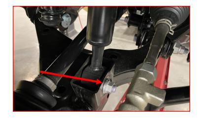
Remove the four (4) upper strut bolts.
