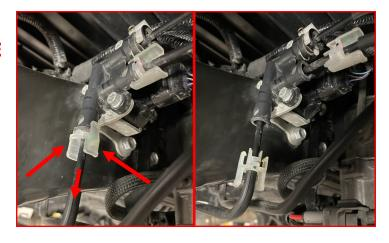
Using two small picks or flathead screwdrivers, **carefully** separate the tabs from the airline hose and pull the hose out of the fitting. Let it hang out of the way. Repeat on the other connector.
