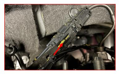
Using factory hardware, attach the factory ABS bracket to the strut tower.
