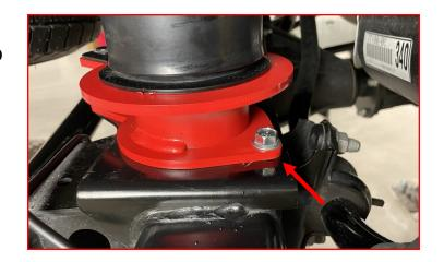
Use the supplied M10-1.25 serrated flange nut to attach it to the axle.
