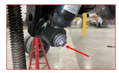
Remove the upper shock nut and bushing.
