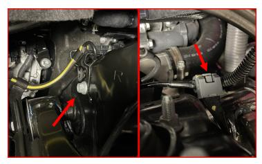
Using factory hardware, raise the lower control arm enough to install the lower strut bolt.
