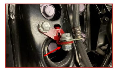
Attach the upper control arm ABS wire bracket to the upper control arm stud using the supplied M8 locking nut and M8 washer.
