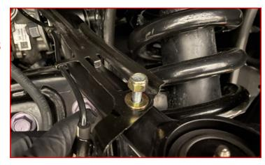
Using factory hardware, attach the ABS sensor wire at the middle of the knuckle.
