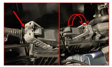
Release the hose clip on the middle plug by pressing in on the tabs on both side and lifting up.
