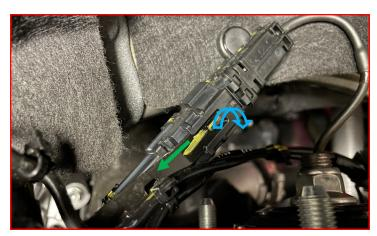
Using a small screwdriver or pick, carefully release the six (three on each side) latches on the plug while prying open the plug.
