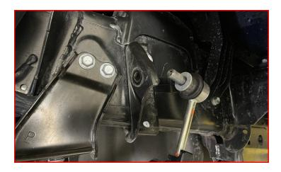
Remove the Panhard bar bolt at the axle and let it rest in the mounting perch.
