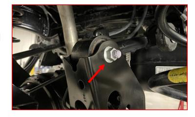
Loosen but **DO NOT** remove the lower control nut at the axle.
