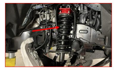
Install but **DO NOT TIGHTEN** the factory lower strut hardware.
