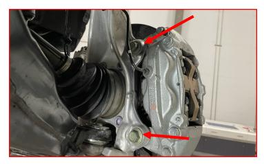
Remove the factory bump stop by unscrewing it from the chassis mount.
