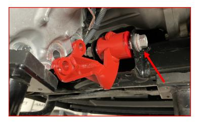
Install the supplied M14-1.5 x 60 SHCS and M14 flat washer into the upper differential mounting hole.
