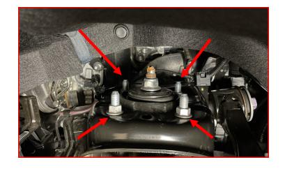
Loosen but **DO NOT** remove inner control arm nuts.
