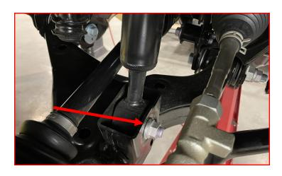
Remove the four (4) upper strut bolts.
