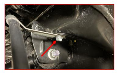
Remove the **bolt** holding the brake line to the frame.
