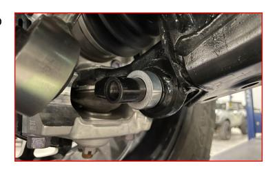
Torque the sway bar end link factory hardware to 80 ft-lbs.
