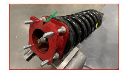
Place the strut and spacer assembly into the control arm.
