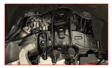
Install ReadyLift front strut spacer onto the strut using factory hardware.
