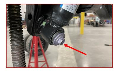
Remove the upper shock nut and bushing.
