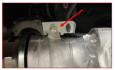
Relocate the bracket from the bottom on the mounting point to the top of the mounting point and attach using the factory hardware.
