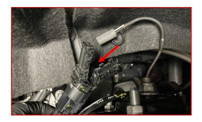
Close the latch on the plug until all six (6) latches click into place.
