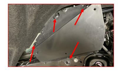
Remove the four (4) clips for the front dust shield
