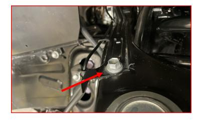
Remove the brake line from the bracket on the chassis.
