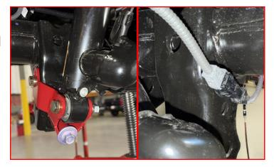
Use an airline to gently inflate and seat the air bag against the axle mount. Install the oe retaining nut.
