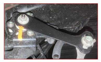
Attach the ball stud to the sensor arm near the same location in the slot as the OE orientation.
