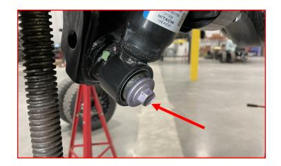
Remove the upper shock nut and bushing.
