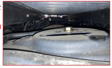
Slide the ReadyLIFT lower shock extension over the factory shock mount boss and install the factory bolt.
