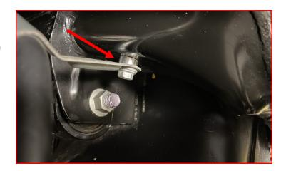
Using factory hardware, install the rear brake line relocation bracket holding the brake line to the frame.
