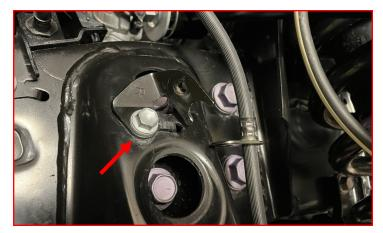
Using factory hardware, install the ReadyLift brake line bracket.
