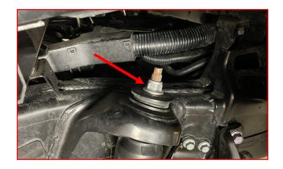
Remove the lower shock bolt and pull the shock free from the shock mount.
