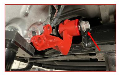
Install the supplied M14-1.5 x 60 SHCS and M14 flat washer into the upper differential mounting hole.
