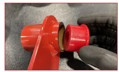
Press the supplied crush sleeve into the bushings and slide the spacers over the sleeves. The sleeve should be about flush with the spacers.
