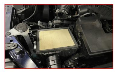
Slide the air box lid into the intake hose and clip it to the air box.
