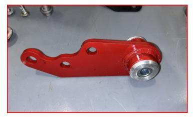
Using factory hardware, attach the ReadyLIFT driver diff drop bracket to the chassis.
