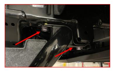
Remove the sway bar end link bolt from the lower control arm and slide the end link off of its perch.
