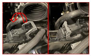
Plug the center plug into the accumulator and lock it in place by closing the handle to the right.
