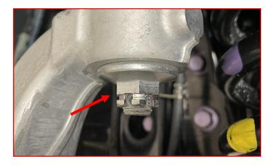
Use the appropriate tool to release the taper on the upper ball joint.
