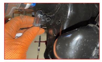
Reroute the wire to the opposite side of the shock mount and insert the clip into the hole.
