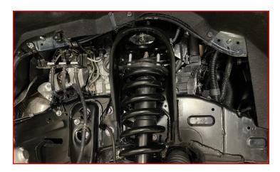
Remove the lower strut bolt and let the strut rest in the lower control arm.
