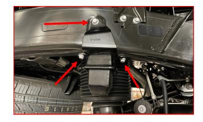
Using the supplied M8-1.25 x 40 hex head flange bolt and the aluminum crush sleeve, attach the bump stop extension to the frame using the top hole on the extension.
