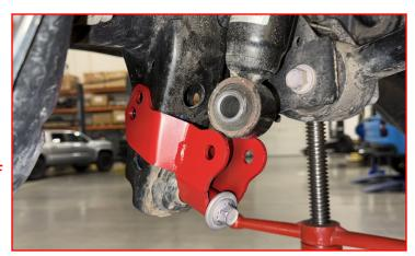
Install the supplied M12 x 75 mm bolt and washer through the shock extension and shock mount. Thread the M12 nut and washer on the inside of the shock mount.
