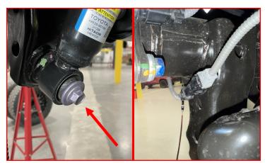
Remove the **nut** securing the air bag to the axle housing.
