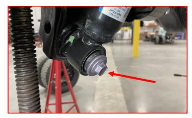
Remove the three bolts holding the factory bump stop to the frame.
