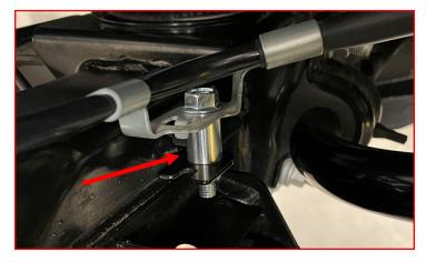
Install the rear brake line spacer—short between the brake line and the chassis using the factory bolt (one on each side) holding the brake line to the axle.
