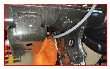
Rotate the shock such that the AVS solenoid is facing away from the axle housing.
