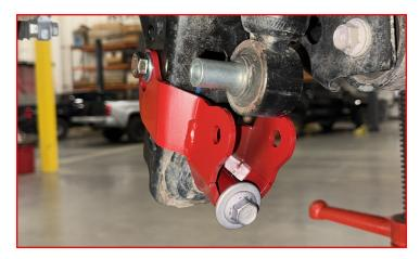
Raise the axle enough to install the supplied M12x75mm bolt, nut and washers through the shock extension and shock.
