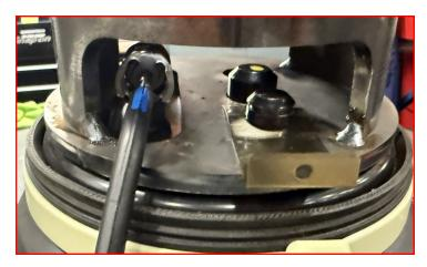
Insert the bag and spacer into the vehicle. Use the supplied M14-2.0 bolt and washer to secure the assembly against the frame.
