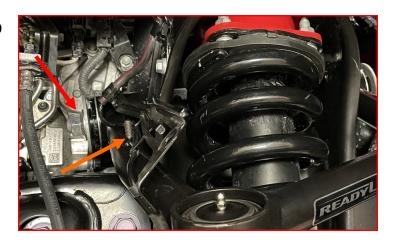
Lower the upper control enough to insert the ball joint stud into the knuckle. Use the supplied M12-1.75 lock nut and stepped washer.
