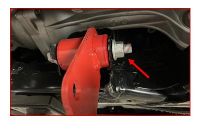
Attach the diff drop bracket to the differential using factory hardware, supplied M16 flat washers, and M16-1.5 C-lock nuts. Note the orientation of the hardware.
