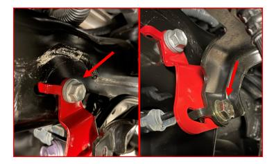
Install the bracket holding the brake line to the axle using factory hardware.
