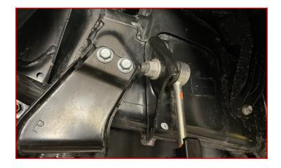
Equally tighten the factory Allen head bolts until they are all snugged against the housing.
