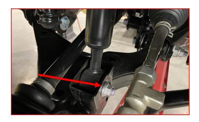
Remove the four (4) upper strut bolts.
