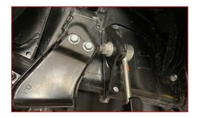
After compressor activates and fills the air bags, loosen the ball stud and adjust the arm to achieve desired ride height.
