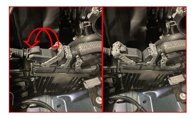
Plug the electrical plug back into its housing.
