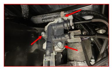
Loosen but **DO NOT** remove the lower shock bolt.
