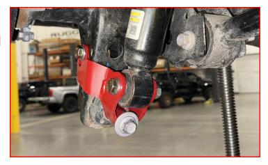
If vehicle is equipped with AVS, remove the harness clip from the shock mount.
