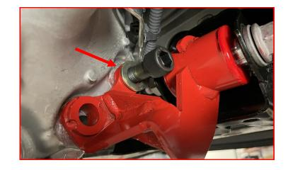
Install the factory hardware (driver side differential bolt) into the lower hole.
