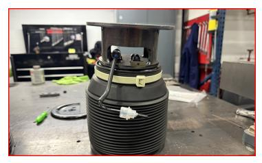
Use the OE retaining clip to secure the bag to the spacer during assembly.
