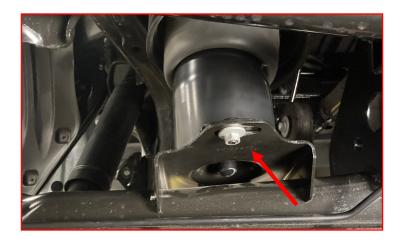
Once the air is released from the bags, remove the spring clip on the top of the bag between the bed and frame rail.
