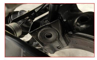
Lower the control arm enough to remove the strut assembly.
