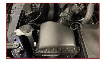
Plug the MAF sensor back into its housing.
