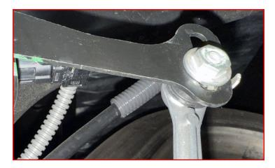
Use the OE hardware to replace the OE sensor arm with the supplied sensor arm.
