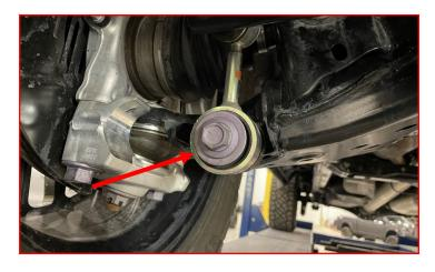
Torque the sway bar bracket factory hardware to 80 ft-lbs.
