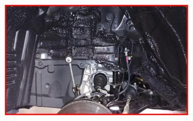
Install the ReadyLIFT strut extensions to the strut using the provided M10 flange nuts. Torque to 30 ft-lbs.
