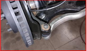
Install the ABS and brake line brackets to the knuckle in the same order they were removed using the factory hardware. Torque to 5 ft-lbs. Install the ABS wire into the plastic clip.
