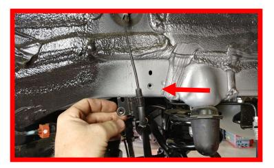
Under the driver side locate the fuel filler shield. Remove the 2 nuts and one plastic rivet. Set cover aside.
