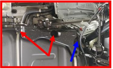
Support the rear suspension cradle using a suitable jack.
