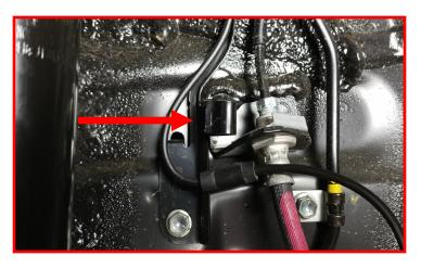
Remove the ABS wire and brake line bracket from the strut body. The ABS bracket sits in front of the brake line bracket. Open the plastic clip on the strut to remove the ABS wire from this point. Let all hang out of the way. Remove the brake line bracket at the knuckle.
