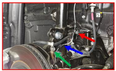
Remove the tie rod end nut. Strike the tie rod end boss with a dead blow hammer to dislodge the taper. Let hang out of the way. This allows you to turn the knuckle free of the rack and pinion to remove the strut.
