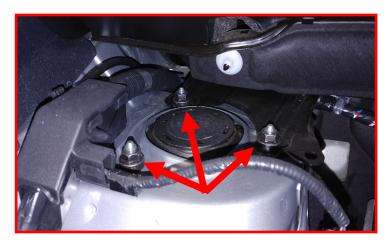
Remove the strut from the vehicle. Be careful to not dislocate the cv shafts from their housings. If this happens, carefully push the CV axle back into the cup. You may have to rotate the hub at the same time.
