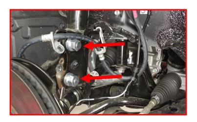
Install the tie rod end to the knuckle using the factory hardware. Torque to 65 ft-lbs. Line up the cotter pin hole with the slots in the castle nut. Install the cotter pin.
