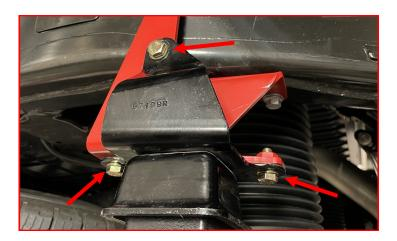
Raise the axle and tighten the upper shock hardware.
