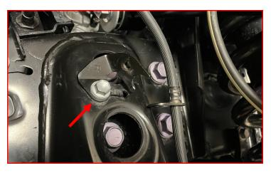
Using factory hardware, install the ReadyLift brake line bracket.
