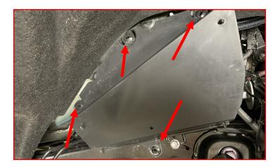
Remove the four (4) clips for the front dust shield
