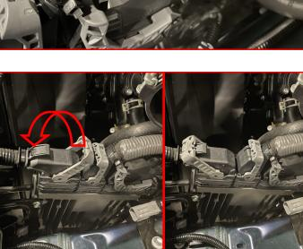
Slide the air box lid into the intake hose and clip it to the air box.
