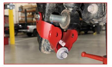
Install the supplied M12x75mm bolt, nut and washers through the shock extension and shock.
