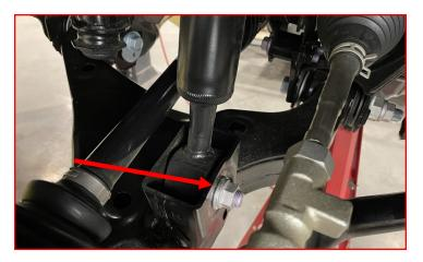
Remove the four (4) upper strut bolts.
