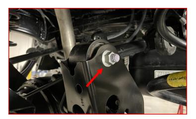
Loosen but **DO NOT** remove the lower control arm nut at the axle.
