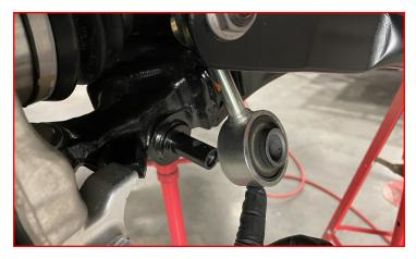
Remove the ABS wire bracket on the upper control arm.
