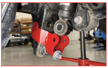
Install the supplied M12 x 75 mm bolt and washer through the shock extension and shock mount.
