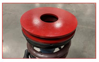
Insert the spring onto the axle.
