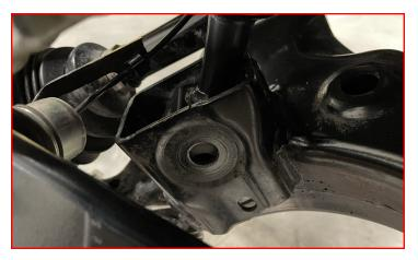
Lower the control arm enough to remove the strut assembly.
