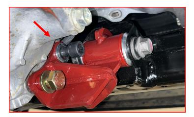
Install the supplied M14 flat washer and M14-1.5 x 60 Hex Head Bolt into the lower hole.
