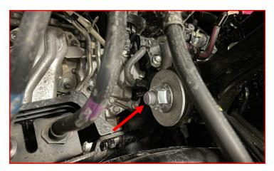
Remove the upper control arm bolt and remove the upper control arm.
