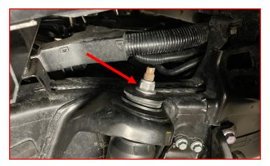
Remove the lower shock bolt and slide the shock off the shock mount boss.
