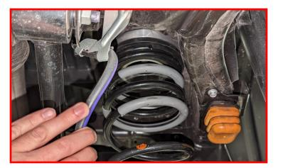
Raise the axle in order to retain the springs in the vehicle. Raise the axle enough to re-install the lower shock bolt.
