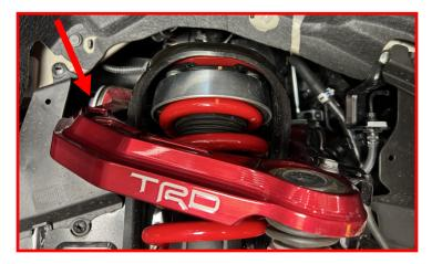
Remove the two bolts holding the lower ball joint cradle to the knuckle.
