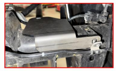
Align the rear bumps top pad hole with the brake line bracket axle mount on the backside of the axle housing.
