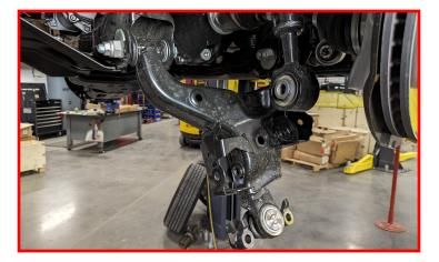
Remove the four (4) upper strut bolts and remove strut from vehicle.
