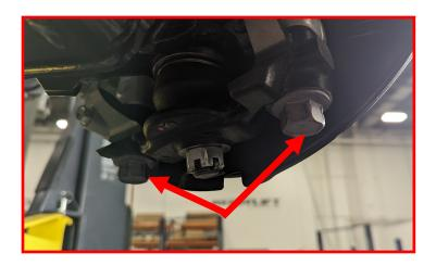
Remove lower control arm to strut bolt.
