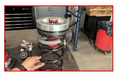
Install spring assembly into the vehicle.
