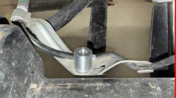
Install the appropriate bump stop pad on top of the axle housing and bump pad spacer.
