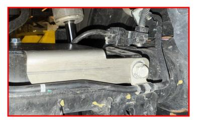
Install the supplied M8x40MM bolt and washer through the bump pad, bump pad spacer, ABS bracket and into the axle mount.
