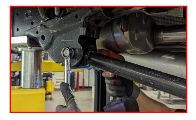
Disconnect sway bar link from sway bar. **RETAIN FACTORY HARDWARE.**
