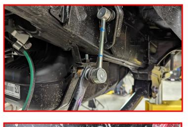
Remove factory bump stop and bracket from vehicle.
