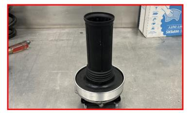
Re-install the top hat with the preload spacer, the isolator and the dust boot. Ensure that the mark made in the previous step aligns with the mark on the spring.
