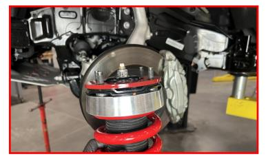
Install the strut assembly back into vehicle using the factory nuts.
