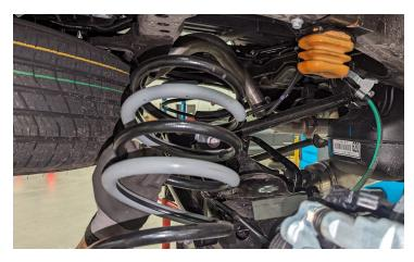
Remove the isolator from the spring.
