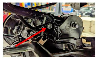
Install sway bar link into sway bar.
