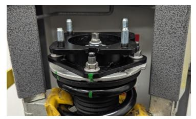
Remove the top hat, spring isolator and dust shield from the assembly. There is a jounce bumper inside the dust boot. Ensure that the jounce bumper remains with the top hat assembly throughout this process.
