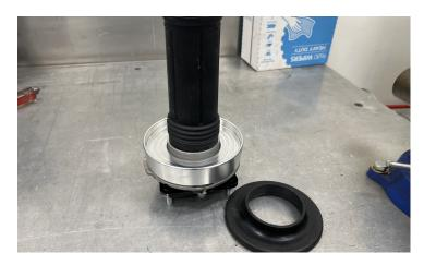
Install the spring isolator into the assembly.
