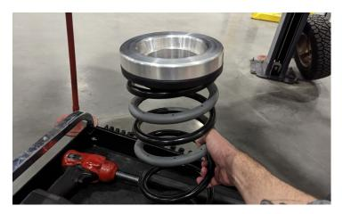
Install spring assembly into the vehicle.
