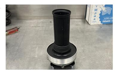
Re-install the top hat with the preload spacer, the isolator and the dust boot and rotate the top hat and ReadyLIFT front strut spacer so that the mark made in the previous step aligns with the mark on the spring.
