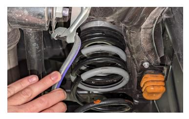
Raise the axle in order to retain the springs in the vehicle. Raise the axle enough to re-install the lower shock bolt.
