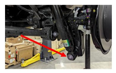
Loosen, but DO NOT REMOVE upper shock nut. Ensure axle is supported, and disconnect shock from axle stud.
