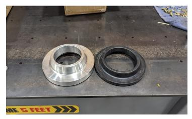
Install isolator onto ReadyLIFT spring spacer.
