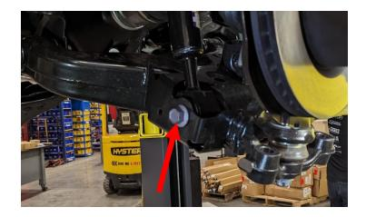
Install the lower ball joint cradle into the knuckle using factory hardware.
