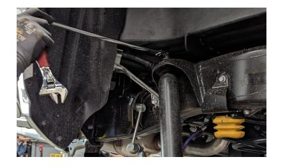
Install bolt into brake line bracket.
