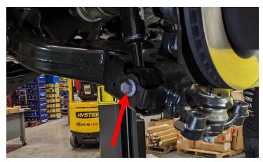
Loosen but **DO NOT** remove inner control arm nuts. Allow the lower control arm to swing out of the way.
