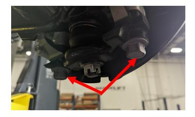
Remove lower control arm to strut bolt.
