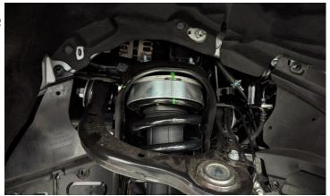
Install the lower strut bolt and nut.
