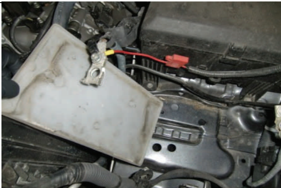
Remove battery and plastic tray from truck .
