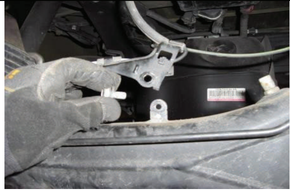
Disconnect ABS wiring brackets from axle.
