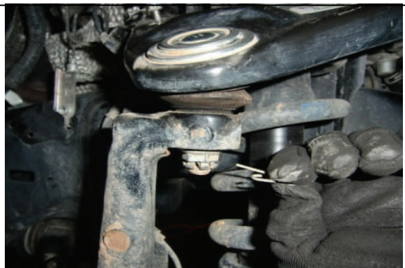
Remove cotter pin and loosen upper ball joint nut.
