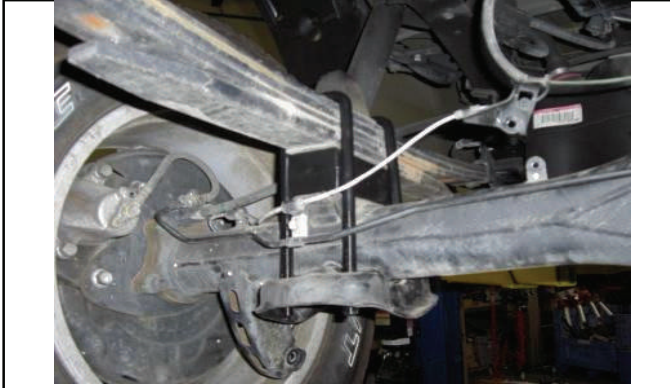
Attach lower mounting plate with provided hardware.
