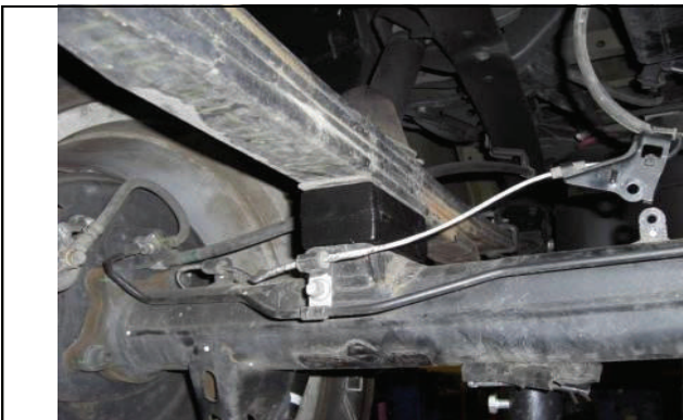
Raise axle and ensure locating pins are properly aligned.
