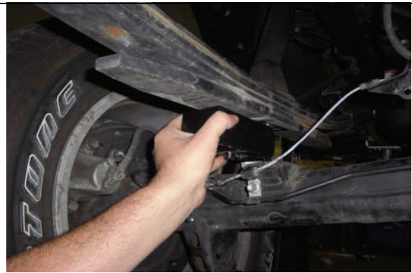
Place new lift block into position between axle and leaf pack.
