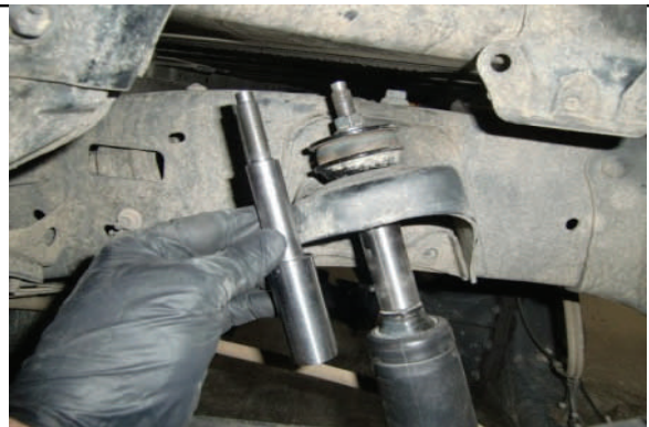
Install provided upper shock extension as shown.
