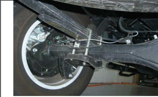
Work on one side at a time to prevent driveline damage.
