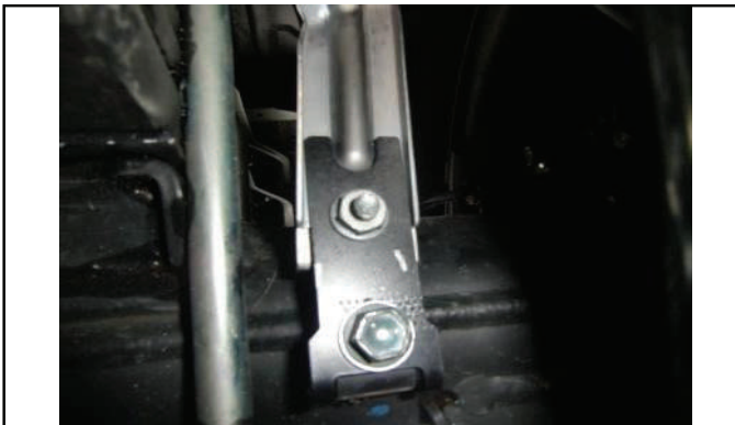
Install provided brackets with OE and provided hardware.
