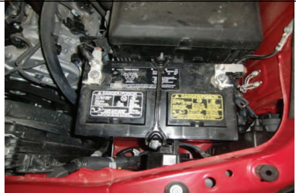
Disconnect positive/negative terminals and hold down clamp.
