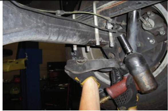
Remove u-bolt nuts and lower plate.
