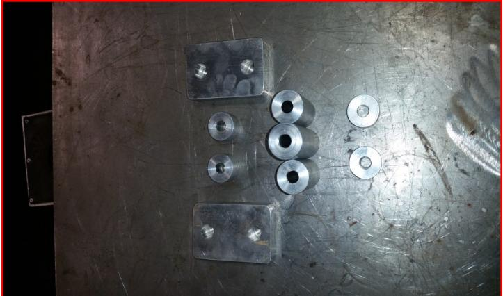
There are 9 billet spacers used on the pro skid plate. 2 rectangular, 4 small round, 2 medium round, and 1 large round. Picture shows placement for the spacers.
