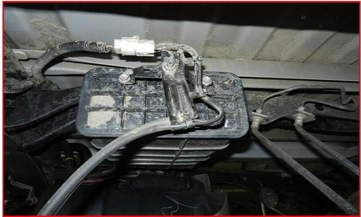
Remove 2 parking brake brackets from the axle.
