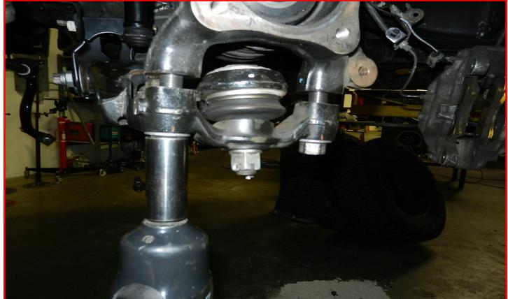
Remove the bump stops from the frame. A large pair of pliers may aid in removal.
