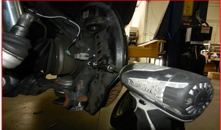
Remove the brake line bracket from the upper control arm.
