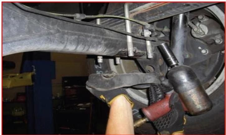
Install the parking brake brackets to the ReadyLIFT extensions using **5/16" x 1" bolts, washers, and c-lock nuts**. Install completed assembly to the axle using **factory hardware**. Torque all hardware to **5 ft-lbs**. Install the ABS bracket to the charcoal canister using the factory hardware. Torque to **5-ft-lbs**.
