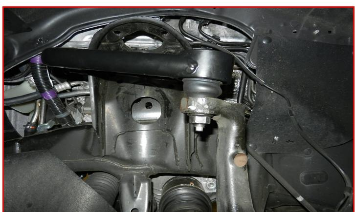
Remove the **lower sway bar end link** from the control arm. Remove the **lower strut mounting bolt**.
