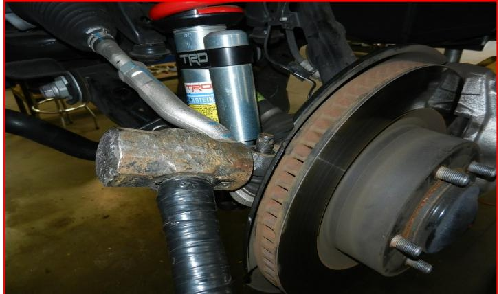
Remove the ABS sensor and harness from the knuckle and hang out of the way.
