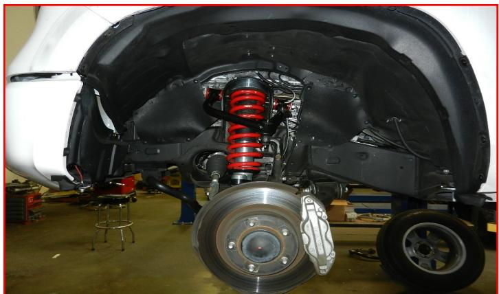
Install the brake line bracket to the ReadyLIFT control arm using the **supplied nut and washer**. Torque to **5 ft-lbs**. Install the outer tie rod end to the knuckle using **factory hardware**. Install the cotter pin. Torque to **65 ft-lbs**. Install the ABS sensor and wire harness to the knuckle using the **factory hardware**. Torque to **5 ft-lbs**.
