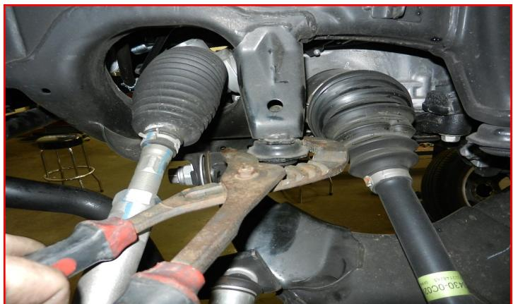
Install the ReadyLIFT bump stop extensions onto the frame and then the factory bump stops to the extensions.
