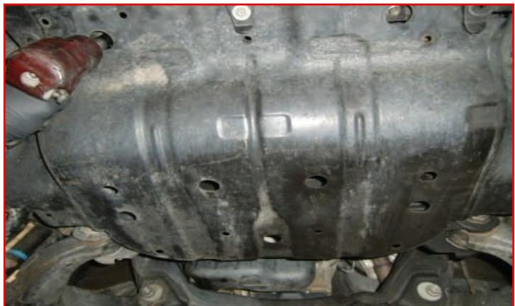
Locate the 2 front differential hanger bolts on the front cross member. Support the differential with a suitable jack and remove these two bolts. Lower the front differential down low enough to install the ReadyLIFT differential drops. Raise the differential up and install to the front cross member using the **supplied hardware**. Torque to **95 ft-lbs**.
