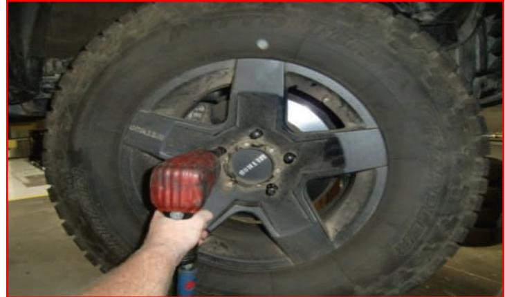
Jounce the front suspension to settle the vehicle to ride height. Center the lower control arm cams and torque to **100 ft-lbs** (**final torque to be done by alignment professional**), upper control arm to **150 ft-lbs**, lower strut hardware to **125 ft-lbs**, and the sway bar end link hardware to **50 ft-lbs**.
