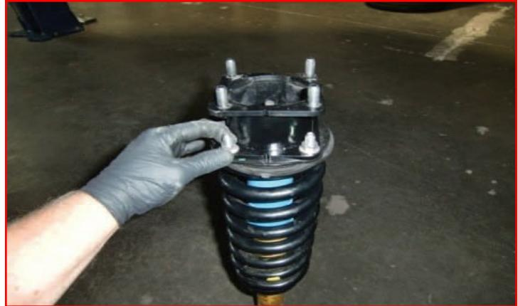
Install the completed strut assemblies into their corresponding sides using the **supplied 10mm nuts**. Do not tighten at this time. It may be easier to only install the nuts closest to the engine bay finger tight so that the struts have some wiggle room to move around while lining up the lower strut bolts. Raise the lower control arm into place and install the lower strut using the **factory hardware**. Do not tighten at this time.
