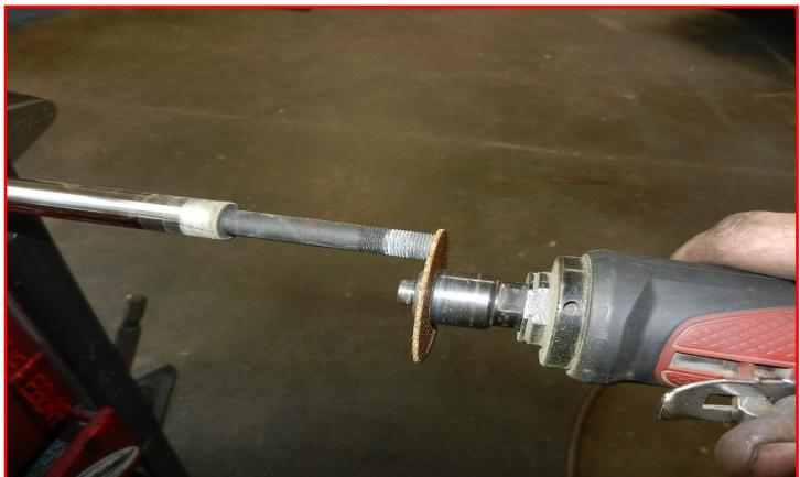
Install the factory crush sleeve that was removed into the ReadyLIFT shock extension. Install the ReadyLIFT shock extension onto the top of the shock, using a liberal amount of thread locker. Install the boot onto the shock.
