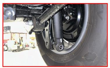
Remove headlight leveling link nut from axle bracket and let the headlight leveling link hang free.
