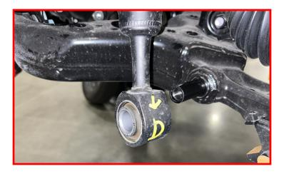
Mark the top hat, spring and lower perch to ensure they are put back together in factory alignment.
