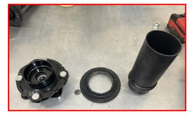
Place the ReadyLIFT Preload Spacer onto the top hat. The ReadyLIFT Logo on the top of the preload spacer should be against the factory top hat.
