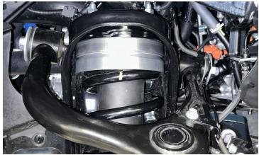
Replace the strut lower mount on the control arm stud and install the bolt.
