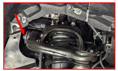
Loosen, but do not remove lower control arm pivot bolts.
