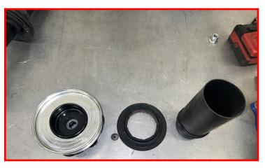
Install the isolator and dust boot into the top hat assembly. Preload spacer should be between the factory top hat and the isolator.
