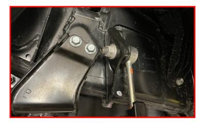
Remove factory bump stop and bracket from vehicle.
