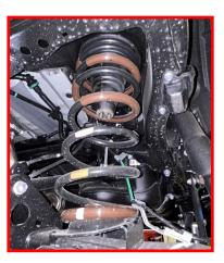
Install ReadyLIFT Spring Spacer on top of spring assembly. Retain factory isolator and bump stop.
