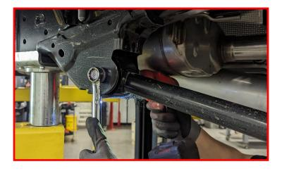
Disconnect sway bar link from frame. **RETAIN FACTORY HARDWARE.**
