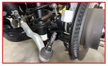
Remove lower control arm to strut bolt.
