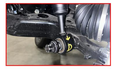
Install the tie rod into the knuckle. Torque nut to 65 ft-lbs. Install cotter pin.
