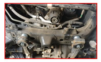
Install the previously removed driver side gravel guard support using the factory hardware. Torque to 45 ft-lbs. (Modified mount shown)
