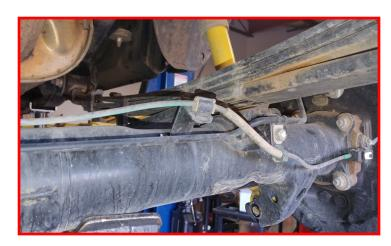
Lower the axle low enough to install the ReadyLIFT block. If the block is tapered, make sure the small end of the block is towards the front of the vehicle. Raise the axle while lining up the center pins. Install the provided u-bolts and hardware. Do not tighten fully, leave loose so that you can repeat the steps for the opposite side. Repeat all steps above regarding the block install.
