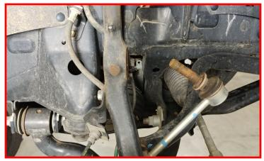
Remove the lower strut hardware.
