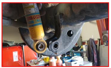
This step is for trucks equipped with 22" or less length rear shocks. Using shock extensions.
