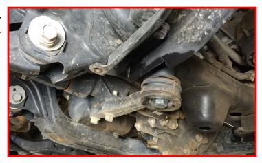
If equipped, install the differential gravel guard to the rear most cross member with the factory hardware and the front cross member with the provided hardware and spacers. Torque to 5 ft-lbs. (Driver side shown)
