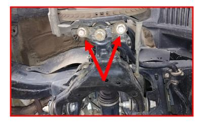
Loosen but do not remove the lower control arm cam bolts. Let the control arm swing down and hang out of the way.
