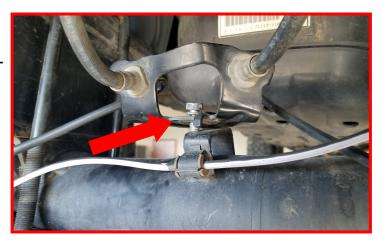
Remove the rear shock from the axle retain hardware.
