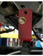
Install the wheels and lower the vehicle to the ground. Torque the wheels to manufactures specifications Jounce the vehicle to settle the suspension to the new ride height. Torque the lower shock hardware to 45 ft-lbs, and the u-bolts to 110 ft-lbs.
