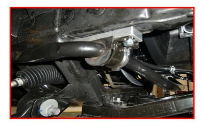
Install the wheels and lower the vehicle to the ground. Torque the lug nuts to the wheel manufacture's specs. Jounce the suspension to get it to settle to the new ride height.
