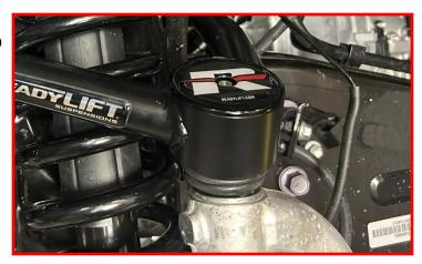
Install the supplied hardened washer onto the ball joint stud.
