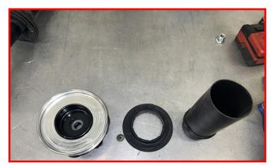
Install the spring isolator and dust boot into the ReadyLIFT preload spacer and top hat assembly.
