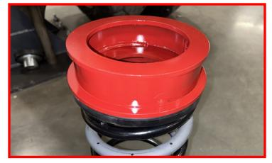
Install spring assembly into the vehicle.
