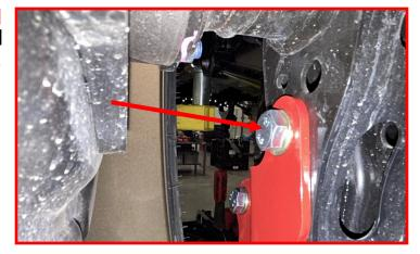
Raise axle enough to install lower shock bolt into rear shock extension.
