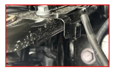
Remove the retaining clip from the upper control arm ball joint nut.
