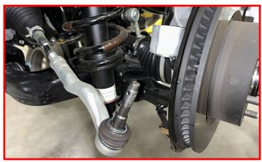
Remove lower control arm to strut bolt.
