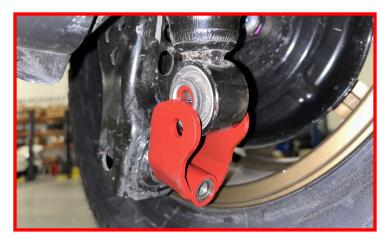
Using the supplied M12 x 30mm hex head bolt, M12 washers and locking nut, install the support tab through the factory shock mount.
