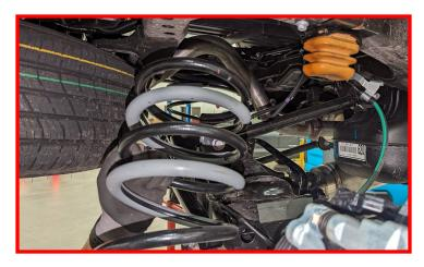
Remove the isolator from the spring. And install isolator onto ReadyLIFT spring spacer.
