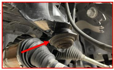
Cut factory bump stop stud down to a length of 0.250".
