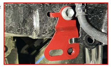
Install rear brake line bracket onto the brake line drop bracket using the supplied M8 x 20mm, M8 flat washer and thread locker.
