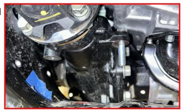
Assemble ReadyLIFT rear differential mount as shown.
