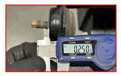
Thread bump stop into bump stop extension until it sits flush against the aluminum.
