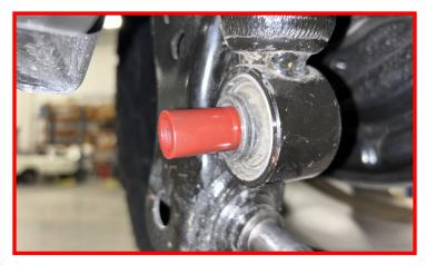
Install ReadyLIFT rear shock extension onto axle.
