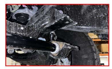
Install the core support nut.
