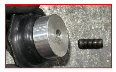
Install stud using internal hex.
