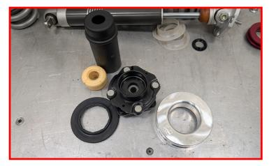
Install the ReadyLIFT preload spacer in between the top hat and the spring isolator. The lip of the preload spacer should be facing away from the top hat, (pointing down in vehicle).
