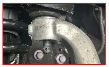
Remove the upper control arm pivot nut.
