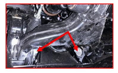
Remove tie rod nut and disconnect tie rod from knuckle.
