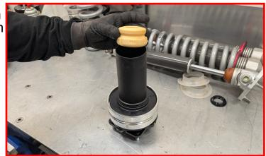
Install the top hat and preload spacer assembly. Rotate the top hat and ReadyLIFT front strut spacer so that the mark made in the earlier step aligns with the mark on the spring.
