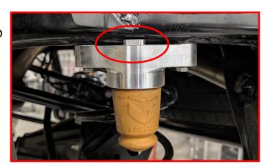
Prior to installing the sway bar you will need to remove the top mounting stud for the sway bar bushing cap.
