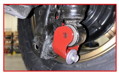
Install the shock into the shock extension using the supplied M12 x 70mm hex head bolt, M12 washers and locking nut.
