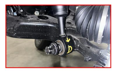
Install the tie rod into the knuckle.
