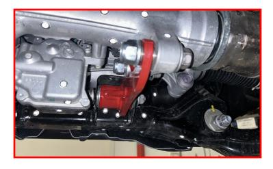
Remove nut holding rear differential mount to frame crossmember.
