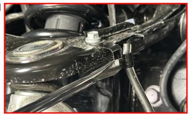
Remove the wire from the bracket.
