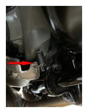
Add the ReadyLift 1" aluminum spacers to the front cradle mounting locations, use the provided hardware M16 bolts, washers, laser cut 2" washer, and the OEM dust shield. Snug these bolts but do not tighten.
