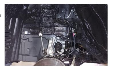
Add the ReadyLift strut spacer to the OEM strut, there is a dot on the OEM strut assembly align the notches on the spacer with this dot. Use the provided hardware M10 flange nuts to secure the spacer to the strut. Torque to 30 ft-lbs. This Alignment is very important for camber correction.
