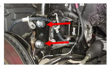
Remove the 3 upper strut mount hardware on the strut tower in the engine compartment. Use of a helper is recommended to hold the strut while removing from the strut tower.
