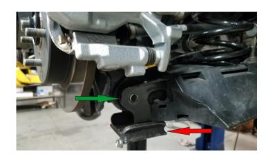
Add the ReadyLift spring spacer to the top of the spring. Use the ruber isolator between the spring and spacer.
