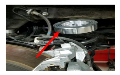
Reposition the spring assembly, so the spring spacer nipple aligns with the hole on the vehicle frame.
