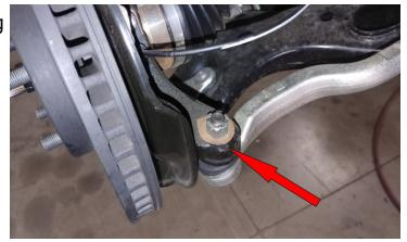
Attach the ABS wire and the brake line to the strut bracket in there original location using factory hardware torque to 10 ft-lbs.
