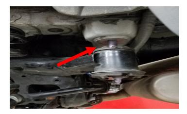
Add the provided 1" step stud to the existing cradle bracket stud. Torque to 19ft-lbs.
