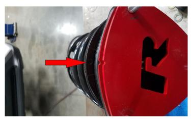
Install the completed strut assemblies into the strut tower using the factory hardware. When installed the R logo so that it is legible from the wheel. Do not tighten at this time.
