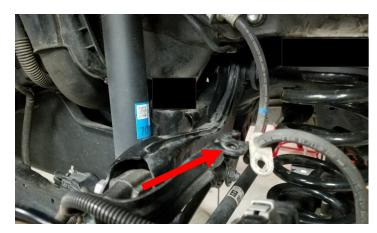
With the suspension cradle supported, remove the front two cradle bolts, dust shield bracket, and the rear cradle nuts. Lower the cradle 1"using the rear cradle studs as an alignment guide.
