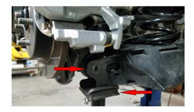
Reattach the brake line using the factory hardware torque 10 ft-lbs.
