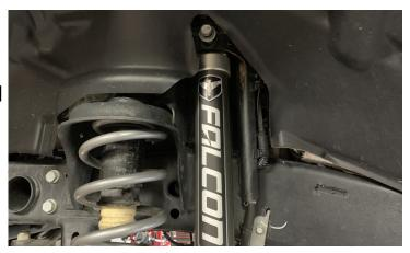
Install the 11" replacement end links to the sway bar using supplied 1/2" bolt, fender washer, flat washer and nut on the sway bar. Be sure to install the fender washer to the outside of the end link. Install the axle side of end link using factory hardware. Torque to 45 ft-lbs.
