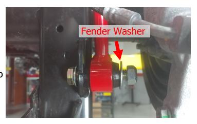
Attach the ReadyLIFT brake line bracket to OE bracket using the provided 1/4" x .75" bolt, washers and nut. Gently rotate/bend the metal brake line. Install using the factory hardware. Torque all to 5 ft-lbs.
