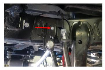
Remove the rear wheel speed sensor and brake caliper, WARNING: Use a hanger to support the caliper, don't let it hang from the brake line or the ABS wire.
