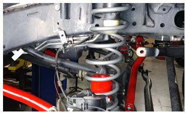
Remove the brake line bracket on the axle for access to install the bump stop nut on the passenger side for bump stop.
