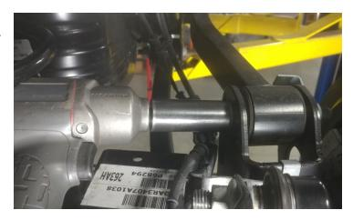
Loosen but do not remove the rear lower control arms at the axle and frame.
