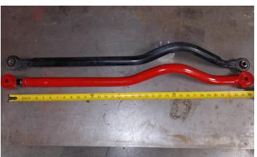
Install adjustable front track bar using the factory hardware.
