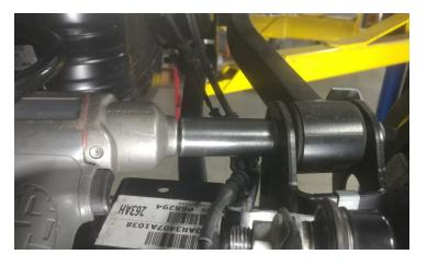
Loosen the rear track bar at the axle and frame.
