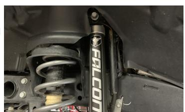
Assemble the 12" straight end links (Add rubber bushing to the end link then add crush sleeve to the bushing.) Install the 12" replacement sway bar end link to the frame using the provided M12 bolt and fender washer. Attach the end link to the sway bar using provided 1/2" hardware do not tighten at this time.
