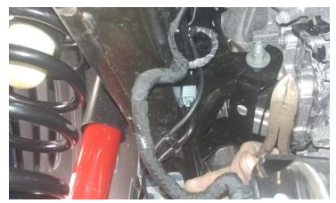
Locate the wire harness on the driver side frame rail and pull all clips out of the frame. Allow the harness to hang out of the way.
