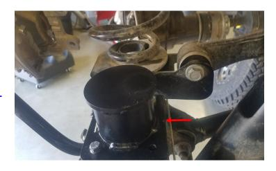
Remove the lower control arms and discard retain factory hardware. Install the replacement lower control arms with the bend facing inboard and the shorter . Do not tighten at this time.
