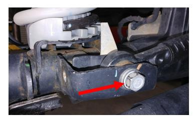
Remove the front track bar bolt at the frame. Retain factory hardware. Remove complete track bar assembly from vehicle and discard.
