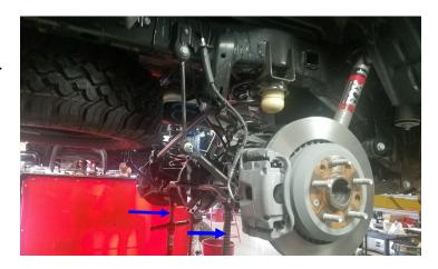
Remove the rear brake line bracket at the frame rail.
