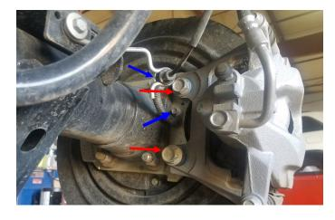
Remove the rear upper and lower shock bolts. Remove factory shock from vehicle and discard. Retain factory hardware.
