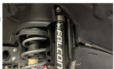
Install the replacement end links to the sway bar using the supplied serrated flange nut on the sway bar. Install the axle side of end link using factory hardware. Do not tighten at this time.
