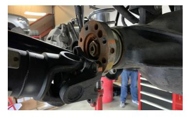
Remove the lower heat shield bolt from the front upper control arm pocket at the frame. Retain hardware for reassembly.
