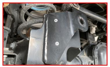
Paint the cut surface to prevent any corrosion.
