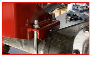
Tighten both the M14 and M12 hardware at this time.
