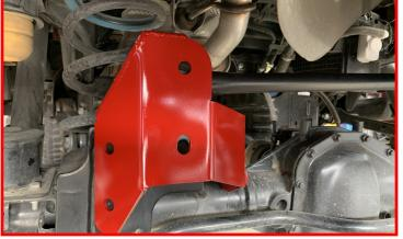
With the track bar relocation bracket on the factory axle mount, mark the (2) 1/2" holes located on the back of the bracket.
