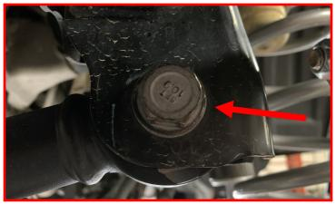
Use caution do not over extend brake lines or wire harnesses. Lower the axle enough to remove the springs.
