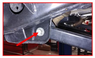
Loosen the front lower control arm hardware at the axle. Do not remove at this time.
