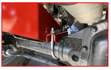
Install the track bar using the factory mounting hardware.
