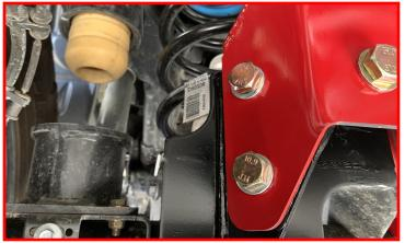
Install the U-bolt around the axle tube and then through the track bar relocation bracket. Start the nuts but do not tighten fully at this time.
