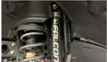
Assemble the 12" straight end links (Add rubber bushing to the end link then add crush sleeve to the bushing.) Install the 12" replacement sway bar end link to the frame using the provided M12 bolt and fender washer. Attach the end link to the sway bar using provided 1/2" hardware do not tighten at this time.
