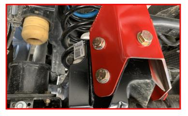
Tighten the U-bolt hardware. Torque the U-bolt hardware to 25 ft-lbs.
