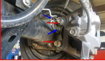
Remove the rear upper and lower shock bolts. Remove factory shock from vehicle and discard. Retain factory hardware.
