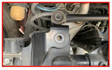
Install the track bar relocation bracket onto the factory axle mount.
