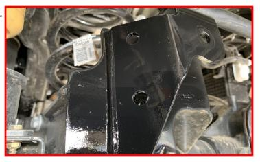
Install the track bar relocation bracket back onto the factory axle mount. Insert the track bar into the relocation bracket prior to sliding the bracket onto the axle mount.
