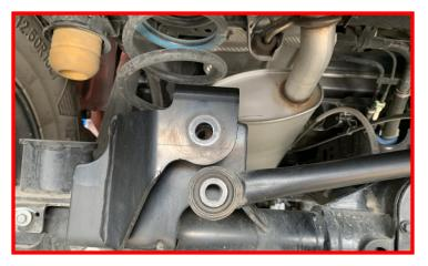
Remove the track bar from the axle mount and swing up and around and place the track bar end on top of the axle mount.
