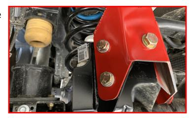
Tighten the U-bolt hardware.
