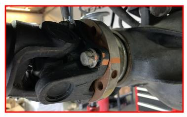
Remove the front drive shaft from differential. Caution do not let the drive shaft hang this may result in damage to the rear seal. Place the drive shaft on top of the differential or use a hanger.
