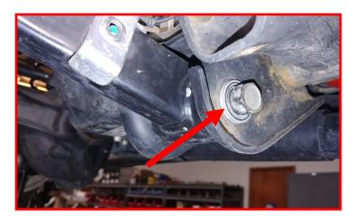
Remove the front shock from vehicle at this point and discard. Retain upper mount factory hardware.
