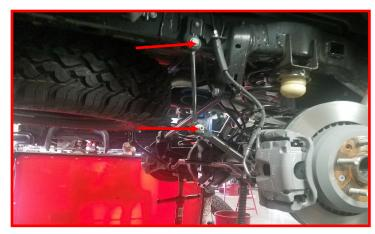
Loosen but do not remove the rear control arms at the axle and frame.
