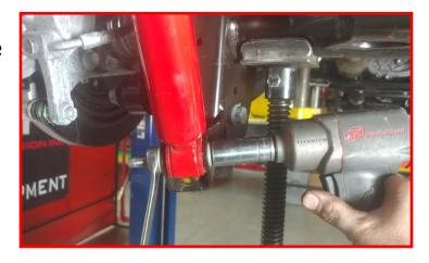
Remove the rear sway bar end link from the axle and sway bar and discard, retain upper factory hardware.
