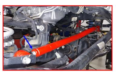
Remove factory front lower control arms at this time and discard, retain factory hardware.
