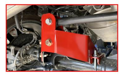
Remove the lower control arms and discard retain factory hardware. Install the replacement lower control arms with the bend facing inboard and the shorter . Do not tighten at this time.
