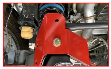
Install the supplied M12 bolt, nuts and washers from the outside of the frame in. Do not tighten at this time.
