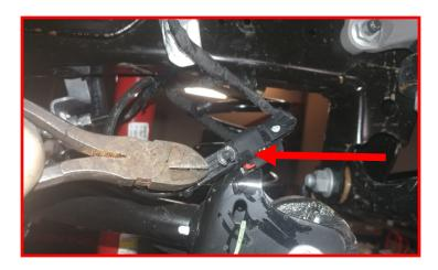
Remove the sway bar end links from the axle. Retain factory hardware.
