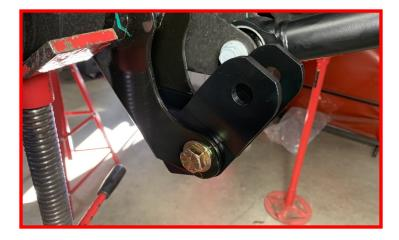
Using an appropriate marker, mark the center of the hole located on the bottom of the rear shock extension.
