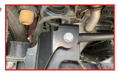
Lower the axle enough to remove the stock spring and rubber isolator.
