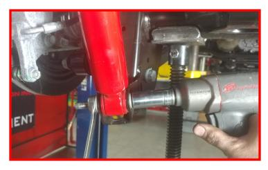
Remove the rear sway bar end link from the axle and sway bar and discard, retain upper factory hardware.
