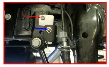
Install the wheels and lower the vehicle to the ground. Torque the lug nuts to the wheel manufacturer specs. Jounce the vehicle a few times to settle the suspension to the new ride height. Torque the upper control arms to 135 ft-lbs, lower control arms and track bar hardware to 135 ft-lbs, shock hardware to 90 ft-lbs and sway bar end link hardware to 50 ft-lbs.
