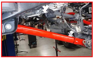
Insert the front bump stop 3/8" x 1.75" Allen bolt into the front bump stop. Insert the front bump stop into the coil spring. Install the coil spring and bump stop at the same time to the frame and axle making sure to clock the spring so that the dead end of the coil sits in the lock on the axle pad. Raise the axle enough to hold the springs in place.
