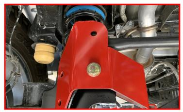
Install the supplied M12 bolt, nuts and washers from the outside of the frame in. Do not tighten at this time.
