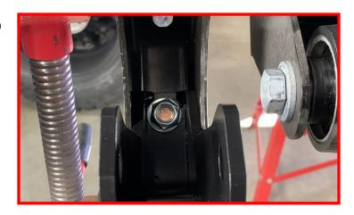
Install the factory shocking into the shock extension using the factory hardware.
