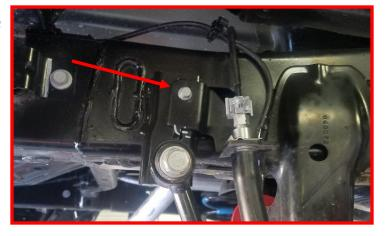
Remove the rear wheel speed sensor and brake caliper, WARNING: Use a hanger to support the caliper, don't let it hang from the brake line or the ABS wire.
