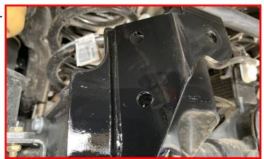
Install the track bar relocation bracket back onto the factory axle mount. Insert the track bar into the relocation bracket prior to sliding the bracket onto the axle mount.
