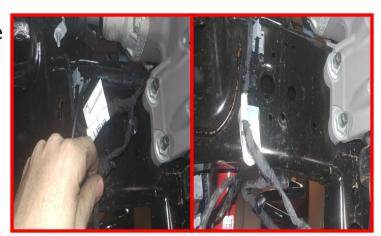
Using a suitable cutting device, clip the outside "Christmas tree" nipple off the electrical connector.
