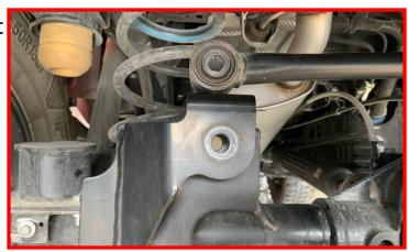
Install the track bar relocation bracket onto the factory axle mount.
