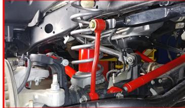
Install the brake line brackets to the lower control arm and frame rail using the factory hardware. Torque to 5 ft-lbs.
