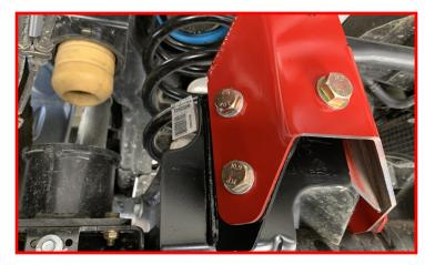
Tighten the U-bolt hardware.
