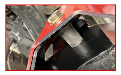
Install the supplied M14 bolt, nut and washers. Do not tighten at this time.
