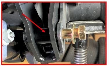
Using the supplied M14 x 70mm bolts, washers and nuts, install through shock extension.
