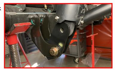
Assemble the 14" straight end links (Add rubber bushing to the end link then add crush sleeve to the bushing.) Install the 14" replacement sway bar end link to the frame using the provided M12 bolt and fender washer. Attach the end link to the sway bar using provided 1/2" hardware do not tighten at this time.
