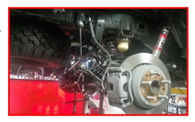
Remove the rear brake line bracket at the frame rail.
