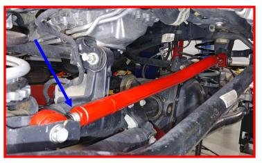
Remove factory front lower control arms at this time and discard, retain factory hardware.
