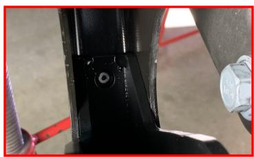
Using an appropriate drilling device. Drill a 1/2" hole in the axle shock mount at the designated hole location marked in the previous step.
