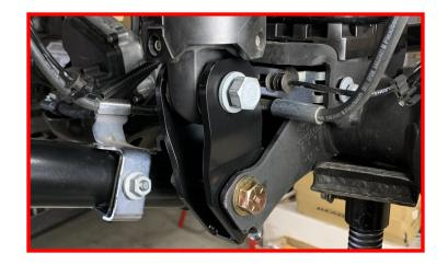
Install the 11" replacement end links to the sway bar using supplied M12 bolt, fender washer, flat washer and nut on the sway bar. Be sure to install the fender washer to the outside of the end link. Install the axle side of end link using factory hardware. Torque to 45 ft-lbs.
