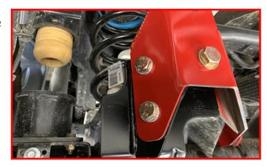
Tighten the U-bolt hardware.
