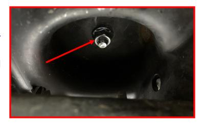
Using a 1/2" drill bit, enlarger the existing hole on the front axle shock mounts.
