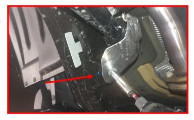
Gently pry the heat shield out of the way and loosen but do not remove the front upper control arm bolts.
