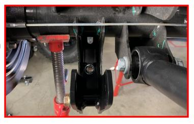
Tighten and torque the M12 hardware to 65 ft-lbs.
