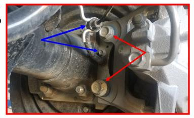
Remove the rear lower shock hardware from the axle mount. Retain the factory hardware
