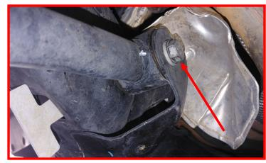
Loosen but do not remove the front upper control arm bolts at the axle.
