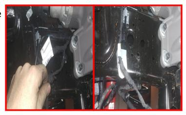
Using a suitable cutting device, clip the outside "Christmas tree" nipple off the electrical connector.
