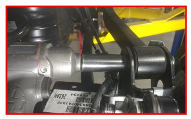
Loosen the frame side track bar mounting bolt.
