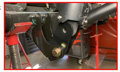
Assemble the 14" straight end links (Add rubber bushing to the end link then add crush sleeve to the bushing.)
