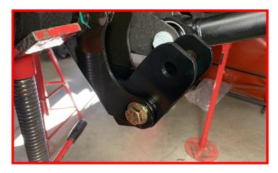
Using an appropriate marker, mark the center of the hole located on the bottom of the rear shock extension.
