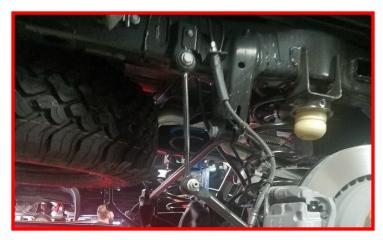
Loosen but do not remove the rear upper control arms at the axle and frame.
