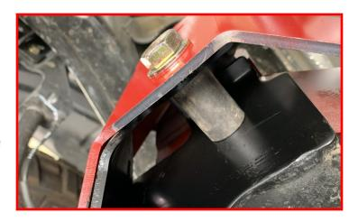
Install the supplied M14 bolt, nut and washers. Do not tighten at this time.
