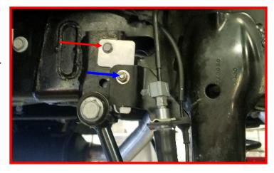
Install the wheels and lower the vehicle to the ground. Torque the lug nuts to the wheel manufacturer specs. Jounce the vehicle a few times to settle the suspension to the new ride height. Torque the upper control arms to 135 ft-lbs, lower control arms and track bar hardware to 135 ft-lbs, shock hardware to 90 ft-lbs and sway bar end link hardware to 50 ft-lbs.
