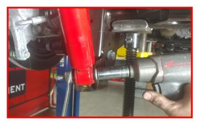
Remove the rear sway bar end link from the axle and sway bar and discard, retain the factory upper hardware.
